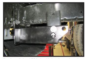
Install the 1/2" bolt with hardware into the rear baseplate hole thru the extension.
