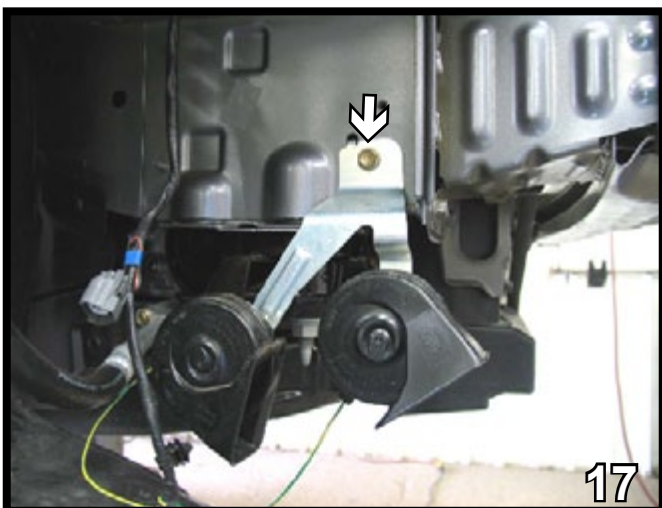
17. Disconnect the horn wiring and, using the 12mm socket, remove one metric bolt from the horn bracket. Set horn bracket and bolt aside to be reinstalled later.
