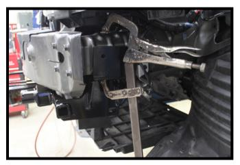
7. Slide the baseplate onto the vehicle, lining up the holes in the baseplate with the existing slots in the frame. Level and clamp the baseplate into position.
