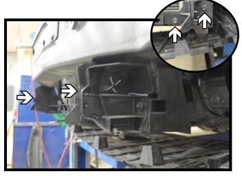
Using a 10MM socket, remove the two (2) screws from air deflector and set aside.
