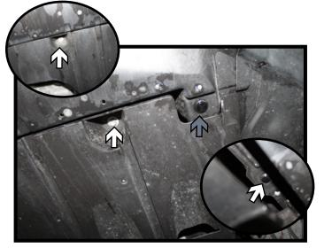
4. Using a 10MM socket, remove the three (3) screws from the front edge of the belly pan. There is one (1) on each side and one (1) in the middle (white). Remove the two (2) push pins from each side (gray). On the backside of the belly pan in the middle, pull down on the plastic shielding behind the pan to expose the push pin underneath (lower inset). Remove this push pin and set the belly pan aside.
