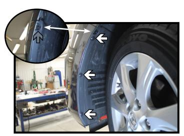
2. Using a Phillips screwdriver, remove the three (3) push pins (white) and the screw (gray) from the outer edge of the wheel well.
