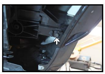
Using a 10MM socket, remove the screw from underside of the fascia. Do this on both sides of the vehicle. Remove the fascia from the vehicle and set aside.
