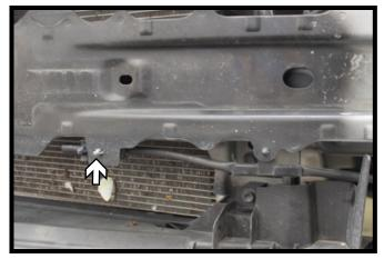
5. Remove the temperature sensor from the bumper and move it aside.
