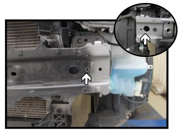
Using a 1/4" drill bit, drill a pilot hole as shown in the bumper. Using a 1-1/4" hole saw, drill out the pilot hole thru the bumper and frame for nut plate access. Do this on both sides of the vehicle.
