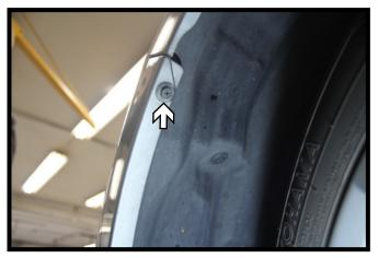
2. Using a 8MM socket, remove the screw from the edge of the wheel well. Do this on both sides of the vehicle.
