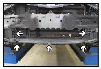
Using a 10MM socket, remove the five
