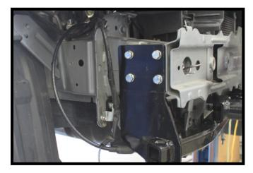
11. Attach the permanent baseplate safety cables to the provided convenience link on the baseplate. The photo shows the recommended installation of the cables to frame of vehicle. Additional options may interfere with suggested mounting; in this case, secure the cables to a solid piece of the frame as described in the instructions included with the permanent baseplate safety cables. Be sure the safety cables do not rub against any hoses or moving parts. Do this on **BOTH** sides of the vehicle.
