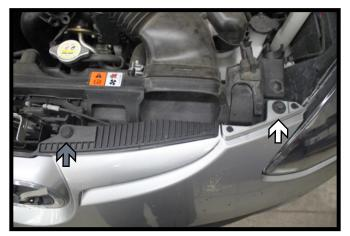
Using a 10MM socket, remove the screw from the top edge of the fascia (white). Then remove the push pin (gray). Do this on both sides of the vehicle.
