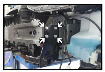
Using a 13/32" drill bit, dril the eight (8) holes on the sides of the baseplate thru the frame. There are four (4) on each side. Install 3/8"-16 x 1-1/4" bolts with 3/8" lock washers into the holes and secure with 3/8" nut plates on the inside of the frame.
