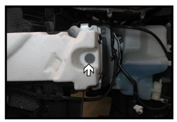
4. Remove the push pin from the styrofoam reinforcement. Do this on both sides of the vehicle. Set the reinforcement aside.
