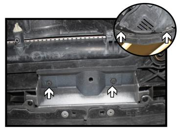
Using a 8MM socket, remove the six (6) screws from the Underside of the fascia. There are two (2) on each side (inset) and two (2) in the middle. Pry the corners of the fascia away from the vehicle. Disconnect all electrical connections and pull the fascia off from the vehicle.
