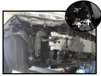
9. Position the baseplate onto the vehicle, start the four (4) 8MM bolts with 5/16" lock and flat washers into the existing frame extension holes (white). There are (2) on each side.
