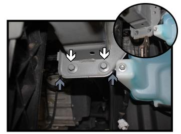
8. Using a 13MM socket, remove the four (4) screws from the lower frame extension. There are two (2) on each side (white). Using a reciprocating saw, cut two (2) slits on the flange back to the face of the frame (gray). Using vise-grips, bend the flange down so it is flush with the face of the frame (inset). Do this on both sides of the vehicle.
