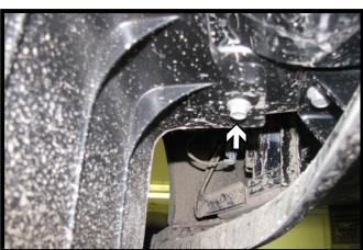
2010-11 Models: Using a 13MM socket, remove the lower air dam from the vehicle. The air dam will not be reinstalled.
