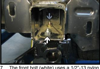
7. The front bolt (white) uses a 1/2"-13 nylon hex nut. The back bolt (gray) uses a 1/2"-13 whiz nut plate. Tighten down while pushing the plate toward the frame. Do this to both sides.
