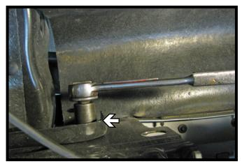
From the top side of the bumper, using a 21MM socket, remove the bolt from inner side of the frame. Do this on both sides of the vehicle.
