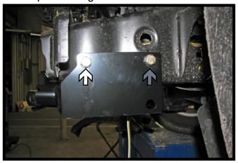
3. With the baseplate as a template, use a 17/32" drill bit to drill the two (2) holes on the sides of the baseplate. Insert a 1/2"-13 x 1-3/4" hex bolt, 1/2" lock washer and 1/2"-13 nylon hex nut into the front hole (white). Then insert a 1/2"-13 x 1-3/4" bolt, 1/2" lock washer and 1/2"-13 whiz nut plate into the back hole (gray).
