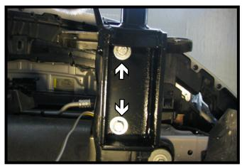
Hold the baseplate up, align with the existing two (2) holes on the bottom of the frame. Insert 1/2"-13 x 1 3/4" bolts, 1/2" lock washers and 1/2" flat washers. Do this to both sides.
