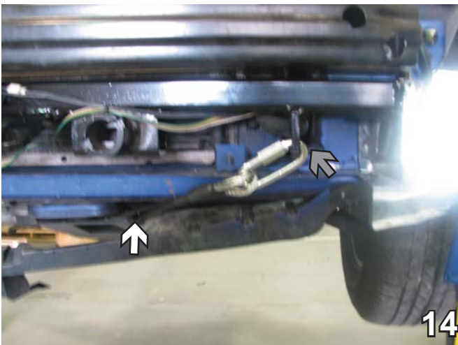
14. Attach the permanent baseplate safety cables to the provided convenience link on the baseplate (see grey arrow). The photo above shows the recommended installation of the cables to frame of vehicle (see white arrow). Additional options may interfere with suggested mounting; in this case secure the cables to a solid piece of the frame as described in the instructions included with the permanent baseplate safety cables. Be sure the safety cables do not rub against any hoses or moving parts. Do this to both sides of the vehicle.
