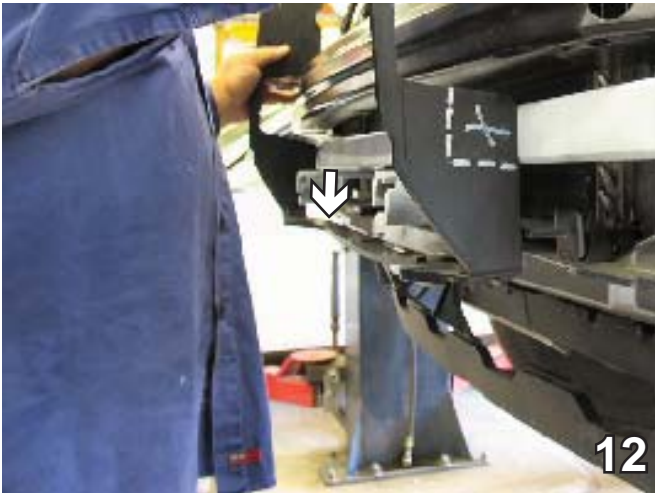
12. Align the air dam as close to the original position as possible, just forward of the baseplate. Mark and trim out area for the air dam and reinstall it to the original position. Note: Baseplate is painted white to increase visibility for instructions only.
