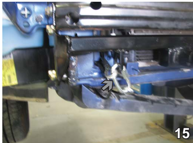
15. On the passenger side, permanent baseplate safety cables are wrapped around twice (gray arrow).
