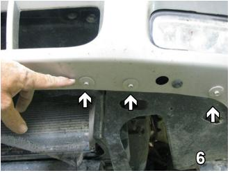
6. Using an 8MM socket, remove the eight screws with washers on the underside of the bumper fascia. Pull the fascia straight out to remove it. Do this to both sides of the vehicle. Set fascia and screws carefully aside to be reinstalled later.
