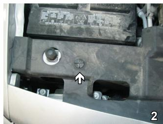
Unscrew three pins from the black plastic on the top edge of the fascia. Lift up and set plastic and pins aside to be reinstalled later.
