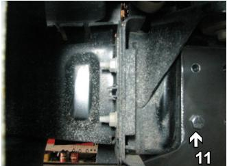
11. Slide the baseplate up on to the frame, then clamp the baseplate securely. Using the baseplate as a template, drill one 13/32" hole on each side. Install and tighten, one 3/8-16 x 1 1/2" hex bolt with a 3/8" lock washer and 14" wire nut plate inserted into the frame. Do this to both sides of the vehicle. Be sure to use loctite on all bolts before tightening.
