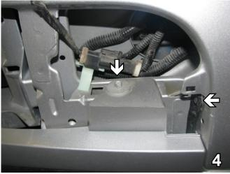
Using the 5MM and 8MM sockets, remove the two hex head screws from blinker opening. Do this to both sides of the vehicle. Set bolts aside to be reinstalled later.
