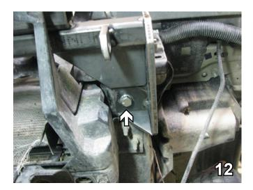
12. Insert one 1/2-13 x 1 1/2" hex bolt with a 1/2" lock washer into the bottom hole and attach it to a 10" wire nut plate inserted into the frame. Do this to both sides of the vehicle. Be sure to use loctite on all bolts before tightening.
