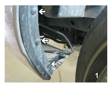
Remove the three Christmas tree pins just forward of the front tire. Do this to both sides of the vehicle. Set the pins aside to reinstall later.
