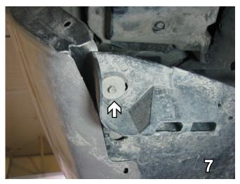
7. Using an 8MM socket, remove the metric screw from the lower side of the air dam. Do this to both sides of the vehicle. Set the screw aside to be reinstalled later.
