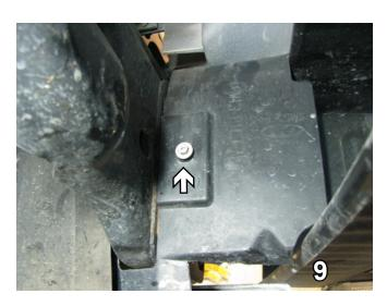
9. Using a 7MM socket, remove one metric screw on the air dam just behind the metal bumper. Do this to both sides.
