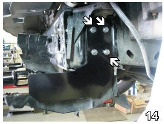
14. Install 3/8-16 x 1 1/2" hex bolts with 3/8" lock washers and 14" wire nut plates inserted into the frame. Do this to both sides of the vehicle. Be sure to use loctite on all the bolts.
