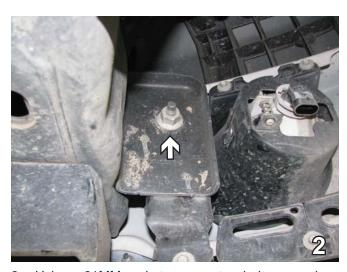
Using a 21MM socket, remove two bolts on each side from underneath the plastic. Do this on both sides of the vehicle. Set bolts aside to be reinstalled later.
