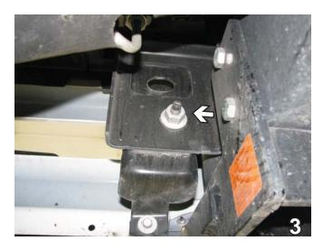
Inside the hood, using a 10MM socket remove one bolt on each side. Set bolts aside to be reinstalled later.
