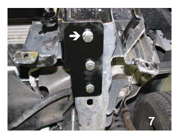
7. Insert 1/2-13 x 1 3/4" hex bolts, 1/2" lock washers and 1/2-13 hex nylon insert lock nuts. Be sure to use loctite. Do this on both sides of the vehicle.
