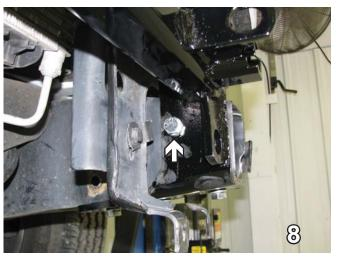
8. On the inside, using the baseplate as a template drill another hole. Attach 1/2-13 x 1 3/4" hex bolts, 1/2" lock washers and 1/2-13 hex nylon insert lock nuts. Be sure to use loctite. Do this on both sides of the vehicle.
