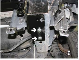
6. Slide the baseplate up, start the two bottom bolts into the existing holes. Use 1/2-13 x 1 3/4" hex bolts with loctite, 1/2" lock washers and 1/2-13 whiz nuts. Using the baseplate as a template, drill the remaining hole (gray arrow). Do this on both sides of the vehicle.
