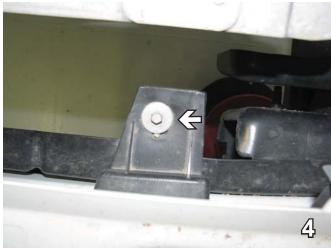
4. Using the 8MM socket, remove three bolts just behind the fascia across the front. Remove the fascia and set aside.
