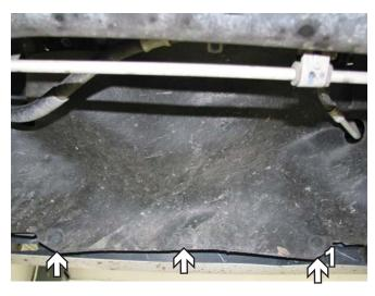
Remove three push pins from underneath the front of the fascia. Do this to both sides of the vehicle. Set the pins aside to reinstall later.
