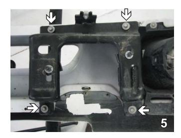
5. On the back side of the fascia, using a 10MM socket, remove the four bolts from the bracket. Do this to both sides. Remount the bracket onto the vehicle for the baseplate to go inside on both sides. Leave the bracket loose until the bumper is back on and in its original position.
