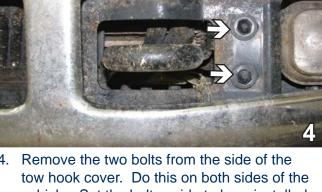
vehicle. Set the bolts aside to be reinstalled later. Some vehicles may need to have the fog lights removed. If so use an 8MM socket to remove the three metric bolts on both sides.
