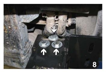
8. Slide the baseplate over the frame rail. Align with the top holes. Insert 1/2-13 x 3 1/2" hex bolts with 1/2" flat washer on the top. Attached to 1/2" lock washers and 1/2-13 hex nuts. Do this on both sides. Tighten with Loctite Red.
