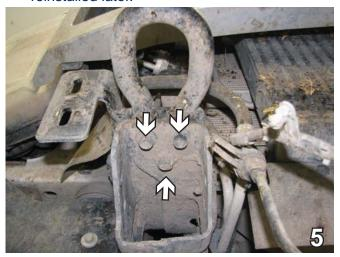
Remove the three 15mm bolts on the underside of the tow hook. Set tow hooks and bolts aside, they will not be reused. Use a 17/32" drill bit to ream the two front holes. Do this to both sides.
