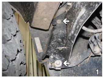
Using a 13MM socket, remove two metric bolts located just forward of the front tire. Do this to both sides of the vehicle. Set bolts aside to be reinstalled later.
