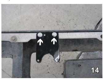
14. Install 1/4-20 x 3/4" bolts with 1/4" flat washers, 1/4 lock washers and 1/4-20 whiz nuts.
