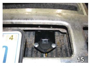
15. Install the electrical plug on the front of the fascia.
