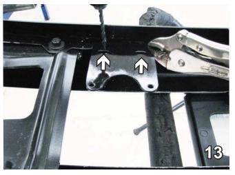
13. Place the metal bumper face down. Position the electrical bracket over the two existing holes on the inside top driver's side. Drill out the hole on the left using a 5/16" drill bit.
