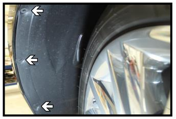
Using a 5.5MM socket, remove the three
