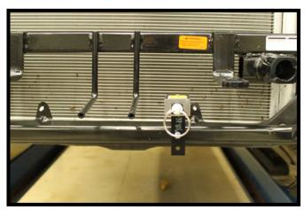
17. **OPTIONAL:** Install the breakaway bracket and breakaway on the driver's side of the vehicle between the convienence link and electrical rods. Drill a 1/4" hole into the frame located below the radiator. Attach the bracket to frame of vehicle with 1/4"-20 x 3/4" bolt and 1/4"-20 nylon nut. Attach the breakaway to the bracket with a 1/4"-20 x 3/4" bolt and 1/4"-20 locking nut.
