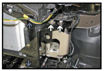
12. Place baseplate on top of frame and line up the holes in the baseplate with the two (2) existing holes on top of the frame. Reinstall the four (4) existing bolts from step 6, two (2) on the top (white) and (2) on the face (gray). Do this to both sides of the vehicle.
