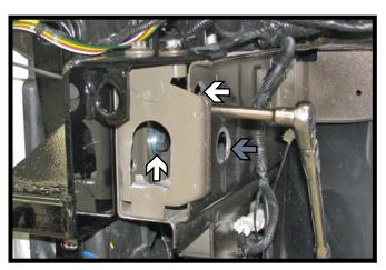
13. Align lower base plate holes to the existing holes. They may need to be reamed out using a 13/32" or 17/32" drill bit. Install a 3/8"-16 x 1" bolt, 3/8" lock washer, 3/8" flat washer and a 3/8" nut w/ wire into the front holes and tighten down (white). Then install a 1/2"-13 x 1" bolt, 1/2" lock washer, 1/2" flat washer and a 1/2" nut plate into rear hole (gray). Do this to both sides of the vehicle.
