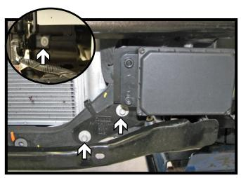
If vehicle is equipped with ACC, on the drivers side only, using an 8mm socket remove the two (2) bolts from the front and the one (1) on the back side of the cruise control box.
