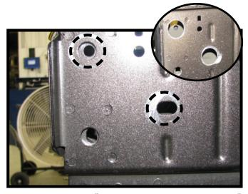
11. Using a 1 1/4" hole saw, drill two (2) 1-1/4" holes into the frame, utilizing the two (2) existing holes in the side of the frame. This gives an access hole to tighten fasteners. Do this to both sides of the vehicle.
