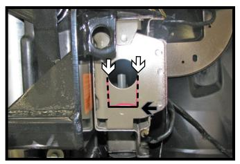
Using a reciprocating saw, make the two (2) vertical cuts (white) to approximately the bend line (black). Bend the cut area into the frame end and as far down as possible. Do this to both sides of the vehicle.
