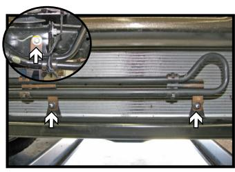
7. On the passenger side front of the vehicle, using a 10MM socket remove the two (2) bolts (white) from the lower coolant line. Then using a 8MM socket, remove the one (1) bolt (gray) located on the side of the vehicle. The lower coolant line now can be swung out of the way.
