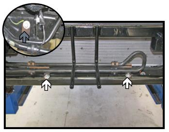
15. Remove coolant line brackets from the back side and relocate to the front of the coolant line. Using the bracket as a template, drill 1/4" holes into the lower cross member and install 1/4"-20 x 3/4" bolts and 1/4"-20 nuts on the back side of the cross member (white).
