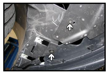
Using a 5.5MM socket, remove the two (2) screws from underneath the front edge of fascia. Do this to both sides of the vehicle.
