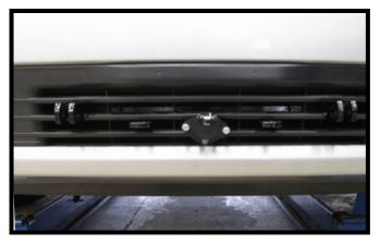
20. Hold the fascia as close to its original position, mark and trim the fascia around the convenience links and attachment tabs. Reinstall the fascia, grill and center panel.
