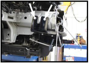
12. Using a 13/32" drill bit, drill the top two (2) holes.
