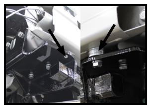
14. Continue using the 13/32" drill bit and drill the bottom, front hole.
