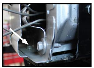
13 . On the driver's side only, use a flat chisel to remove the nut that is located on the outer edge inside the vehicle frame rail.
