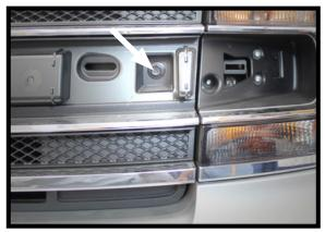
5. Once the center panel has been removed, use a 10MM socket to remove the bolt. There is one (1) on each side of the vehicle.
