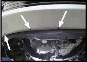
On the underside of the vehicle use a 5.5MM socket to remove seven (7) bolts.
