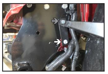
On the driver side, install the attachment plate to the existing tab, using the existing bolt (white). Bend the tab back to it's original position, then connect the air box to the attachment plate with a 1/4"-20 x 3/4" bolt and 1/4" nylon nut (gray). Secure any loose wiring.
