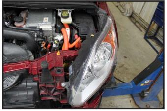
Plug in and reinstall the headlights on both the driver and passenger sides. Secure any loose wiring.
