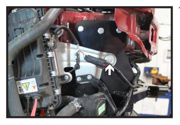
16. **Energi Only:** On the passenger side, reinstall the bracket bolt thru the existing hole in the baseplate.
