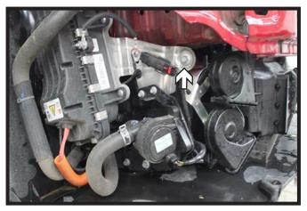
5. **Energi Only:** On the passenger side, using a 10MM socket, remove the screw from the bracket for baseplate installation clearance.
