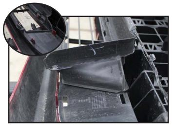
19. Hold the fascia up to the vehicle as close to it's original position. Mark and trim the fascia as needed to clear the baseplate.
