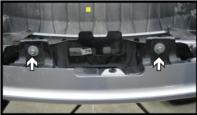
3. Using a 8MM socket, remove the two (2) bolts from the top side of the bumper. Unhook any electrical connections and pull the bumper from the vehicle.
