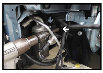
13. Using a 13/32" drill bit, drill the middle hole thru the frame. Install a 3/8"-16 x 1-1/2" bolt with a 3/8" lock washer into the hole and a 3/8" nut plate on the inside of the frame (white). Remove the back bolt, ream out the hole if necessary, reinstall the bolt with a 3/8" lock washer and a 3/8" nut plate on the inside of the frame (gray). Do this on both sides of the vehicle. Tighten all fasteners down.
