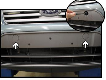
6. Remove the two (2) plastic covers. Then using a T40 Torx, remove the two (2) screws from the fascia. Remove the fascia from the vehicle and set aside.
