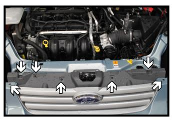
Using a Phillips screwdriver, remove the seven (7) screws from the top edge of the fascia.
