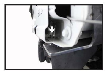
On the driver side bumper, using a chisel or flat screwdriver, remove the nut welded on the inside of the bumper for bolt clearance on step #13.
