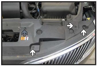
Using a 10MM socket, remove the six (6) screws from the top edge of the fascia.
