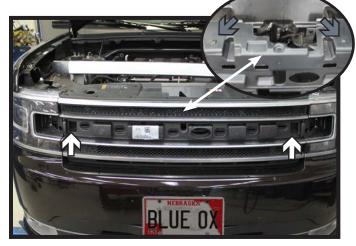
2. Using a 10MM socket, remove the two (2) screws from the face of the grille. Remove the grille from the vehicle and set aside.
