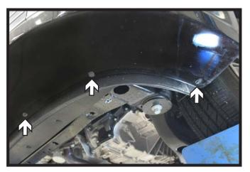
4. Using a 5.5MM socket, remove the screws from the underside of the fascia. Pull the fascia forwards disconnecting all electrical connections and set the fascia aside.
