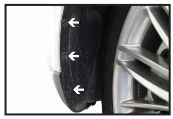
Using a 5.5MM socket, remove the three (3) screws from the outer edge of the wheel well. Do this on both sides of the vehicle.
