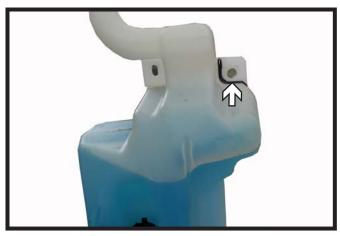
14. Prior to reinstalling the washer reservoir, trim the front mounting tab off as shown.
