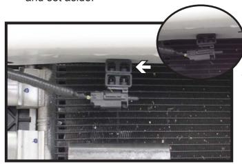
7. On the passenger's side, unclip the air temperature sensor from the bumper.
