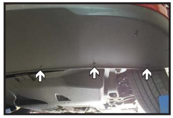
4. Using a 5.5MM socket, remove the seven (7) screws from the underside of the fascia. Pull the fascia forwards disconnecting all electrical connections and set the fascia aside.
