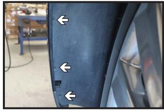
2. Using a 5.5MM socket, remove the three (3) screws from the wheel well. Do this on both sides of the vehicle.
