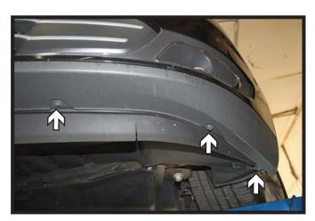
3. Using a 8MM socket, remove the seven (7) screws from the underside of the fascia. There are three (3) on each side and one (1) in the middle.
