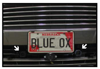
14. Hold the fascia as close to its original position, mark and trim the fascia around the convenience links and attachment tabs. **Important:** Ensure that nothing is installed in front of the ACC sensor. Obstructions will cause false readings from the sensor. Reinstall the fascia.
