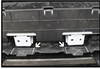
6. Using a utility knife, trim two (2) pockets in the plastic shrouding back flush to the metal brackets as shown.
