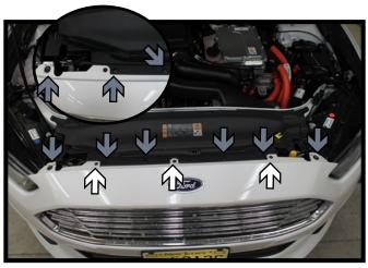
1. Using a T25 Torx, remove the three (3) screws from the top edge of the fascia (white). Remove the six (6) push pins from the top edge of the fascia (gray).
