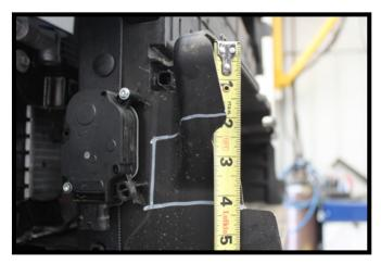
7. Trim the radiator shrouding approximately as shown for baseplate clearance. Do this on three (3) shrouds across the front of the vehicle.
