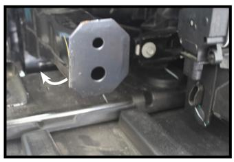
9. Using a hammer, knock the edge of the extension behind for baseplate clearance. Do this on both sides of the vehicle.
