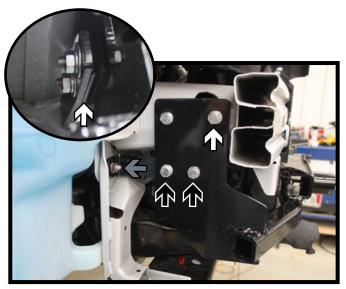
11. Using a 13/32" drill bit, drill the front top hole thru the frame. Install a 3/8"-16 x 1" bolt, 3/8" lock washer and 3/8"-16 nut plate (white). Using a 13MM socket, remove the existing frame nut and install the side bracket with a 8MM flat washer and 8MM nut (gray). Install 3/8"-16 x 1-1/2" bolts, 3/8" lock & flat washers and 3/8"-16 nuts into the lower holes (black) with the spacer plate in between the bracket and baseplate (inset). Do this on both sides of the vehicle.
