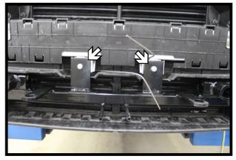
12. Using a 13/32" drill bit, drill the front holes thru the metal brackets. Install 3/8"-16 x 1" bolts, 3/8" lock washers and 3/8"-16 nut plates.
