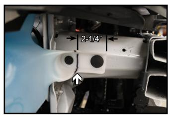
5. Using a utility knife, trim the outer flange of the washer fluid reservoir back approximately 2-1/4"as shown.
