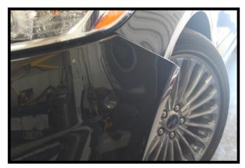
Pull the corners of the fascia out and away from the vehicle. Disconnect all electrical connections from the back side of the fascia. Remove the fascia from the vehicle and set aside.
