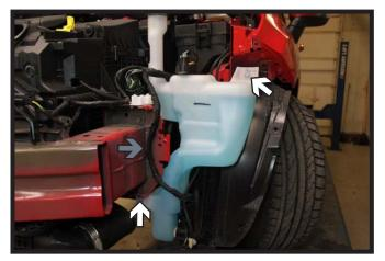
7. Disconnect the wire loom clips from the frame (gray). Using a 10MM socket, remove the two (2) screws from the washer fluid reservoir (white). Disconnect all lines and plug fluid lines. Set the reservoir aside.
