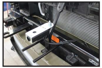
22. **Optional Breakaway:** Install the breakaway bracket to the lower support brace using the existing bolt. Bolt the breakaway to the bracket with a 1/4"-20 x 3/4" bolt and 1/4" lock nut.
