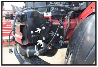
18. Using a 13/32" drill bit, drill the back baseplate holes thru the frame. Bolt the support bracket to the baseplate/frame with 3/8"-16 x 2" bolts, 3/8" lock washers and 3/8" nut plates (white).
