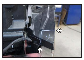
ST/SE Models: Trim the upper shrouding as shown for baseplate clearance. Do this on both sides of the vehicle.
