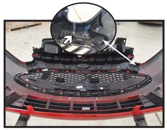
23. On the backside of the fascia, trim off the inner layer of the fascia along the outer groove as shown for baseplate clearance. Do this on both sides of the fascia.
