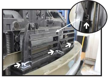
12. **SFE Models:** Using a flat screwdriver, disconnect the back rod from the shutter system (inset).
