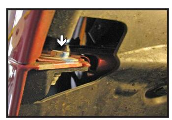
3. Using a 8MM socket, remove the screw from the upper edge of the wheel well. Do this on both sides of the vehicle.
