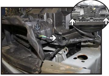
10. **SFE Models:** Remove the four (4) push pins from the shutter shrouding. There is one (1) on each side (white) and two (2) in the middle (inset).
