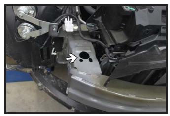
16. Using a 1-1/4" hole saw, drill an access hole on top of the bumper as shown. Do this on both sides of the vehicle.
