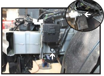
14. SFE Models: On the driver side, using a 8MM socket, remove the two (2) screws from the fuse box. Set the box aside.
