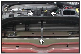
8. Using a 10MM socket, remove the three (3) screws from the latch support brace and pull the brace upwards away from the bumper for baseplate installation.
