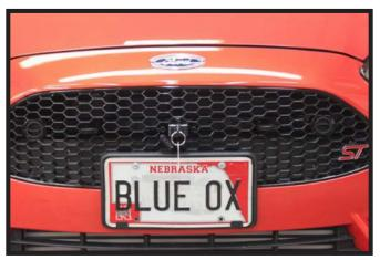
24. Hold the fascia as close to its original position, mark and trim the fascia around the convenience links and attachment tabs. Reinstall the fascia and headlights.
