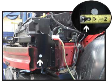
17. Position the baseplate onto the frame, flushing the bottom of the baseplate and frame. Leave a 1/2" gap from the front of the baseplate and the backside of the bumper (inset). Level and clamp into position.
