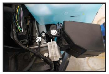
21. **SFE Models:** On the driver side, install the supplied bracket to the frame with the existing bolt. Then the fuse box to the bracket with a 1/4"-20 x
