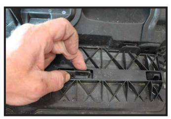
11. **SFE Models:** On top of the shutter shrouding, unsnap the two (2) clips and remove the front section of the shrouding.
