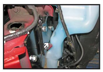
20. Reinstall the washer reservoir. Checking the clearance on the lower part of the reservoir making sure it is not rubbing on the baseplate. It should have minimum 1/16" clearance. If necessary pull the reservoir back and re-tighten the bolts. Reinstall the latch support brace.
