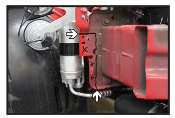
15. Trim the face of the frame extension just below the rib (top arrow) back to the face of the frame (bottom arrow). Do this on both sides of the vehicle.
