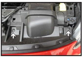
1. Remove the four (4) Phillips head push pins from the top edge of the fascia. There are two (2) on each side.
