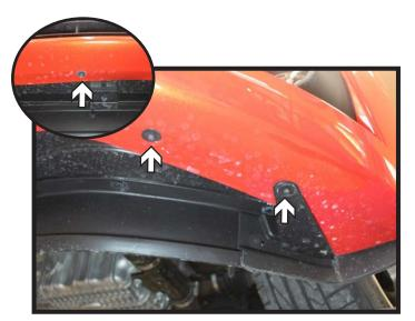
4. Using a 7MM socket, remove the five (5) screws from the underside of the fascia. There are two (2) in each corner and one (1) in the middle.
