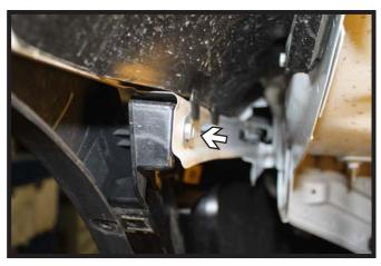
Pull back the fender flare and using a 10MM socket, remove the screw from the inside of the fascia/fender joint. Do this on both sides of the vehicle.
