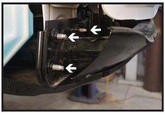
Using a 13MM socket, remove the four (4) bolts from the backside of the crossbar.
