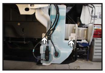
Using a 10MM socket, remove the two (2) screws from the washer reservoir.
