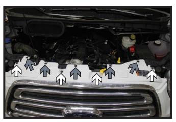
Using a 10MM socket, remove the four (4) screws from the top edge of the fascia (white). Then remove the five (5) push pins (gray).
