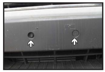
Remove the plugs from the fascia. Then using a 13MM socket remove the two (2) screws from the face of the fascia.
