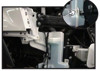
18. Reinstall the washer reservoir onto the vehicle. Use the supplied 1/4" hardware to attach the reservoir to the bracket as shown.
