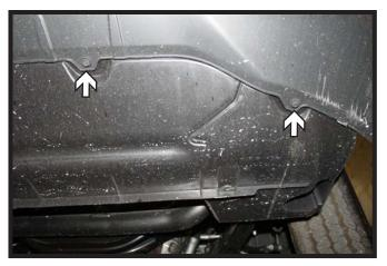
Using a 10MM socket, remove the four (4) screws from the underside of the fascia.
