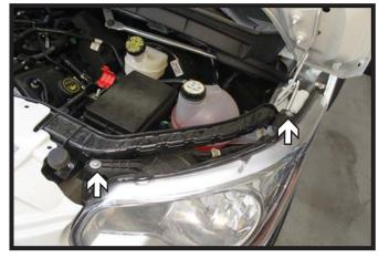
Using a T30 Torx, remove the two (2) screws from the headlight. Disconnect any electrical connections and set aside. Do this on both sides of the vehicle.
