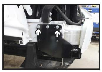
15. Continue drilling the remaing top holes thru the frame with a 3/8" drill bit. Installing 3/8" bolts with lock washers into the holes with a 3/8" whiz nuts on the inside of the frame lip. Do this on both sides of the vehicle. Fully tighten the all hardware.
