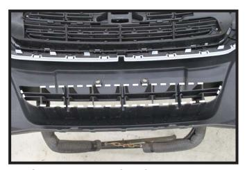
On the backside of the fascia, trim inside grill section out of the lower opening so it is one large opening.
