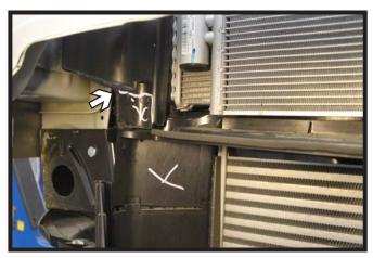
13. Trim the upper section of sheilding just below the bumper and disconnect the lower section. Do this on both sides of the vehicle.
