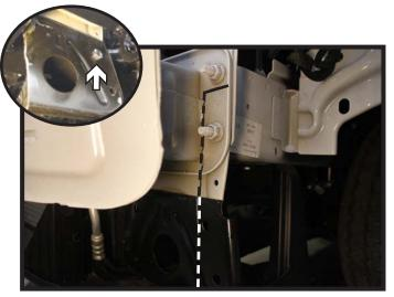
12. Using a reciprocating saw, trim off the frame flange just below the top bolt back to the face of the frame and all the way down. Do this on both sides of the vehicle.
