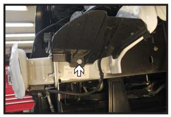
11. On the driver side, using a 10MM socket, remove the screw from the plastic shield. The sheild will not be reinstalled.
