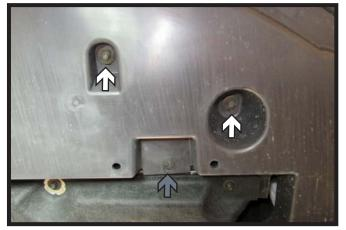
Using a 7MM socket remove the two (2) bolts (white) and one (1) push pin (gray) from the belly pan. Do this on both sides of the vehicle. Remove belly pan.
