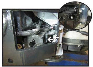
20. Before attaching the safety cables drill out bottom two (2) indicated holes using a 3/8" drill bit. Then insert two (2) 3/8" bolts with lock washers. Do this on both sides of the vehicle.
