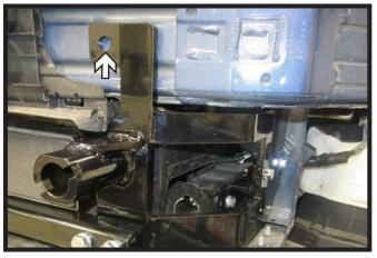
18. Using a 1/2" drill bit drill out top two (2) holes, one (1) on each side. Metal is extremely hard so may need to start with a 1/4" drill bit then work up to a 3/8" drill bit and then eventually use a 1/2" drill bit to create the holes. Make sure to drill slowly.
