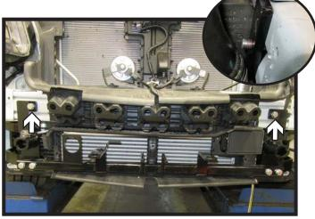
22. Insert 1/2" bolts with spacers on the back side. If the spacer cannot be attached perfectly up and down, may need to angle spacer slightly to get it to fit.
