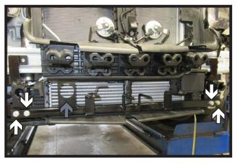
20. Using four (4) 1/2" x 2-3/4" bolts with lock washer and nylon lock nut attach the center cross bar to the side plates. If the holes do not completely line up, ream out holes with a drill bit.
