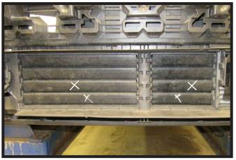
10. Remove the bottom two (2) shutters on the vehicle to allow room for the baseplate.
