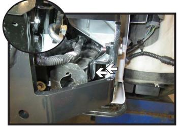
Before attaching the safety cables drill out bottom two (2) indicated holes using a 3/8" drill bit. Then insert two (2) 3/8" bolts with lock washers. Do this on both sides of the vehicle.
