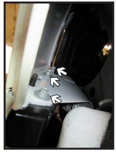
Pull the wheel well liner back and remove the three (3) bolts using a 8MM socket. Do this for both sides of the vehicle.
