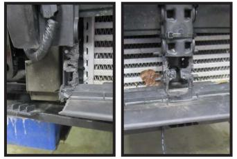
11. Trim the shutter housing on both sides of the vehicle and in the middle as shown to allow room for the baseplate cross member.
