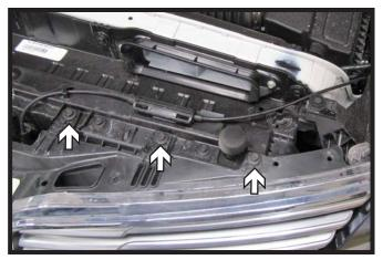
Using a 10MM socket remove the three
