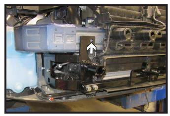
Insert one (1) 1/2" bolt with spacer on the back side. If the spacer cannot be attached perfectly up and down, may need to angle spacer slightly to get it to fit. Do this on both sides of the vehicle.
