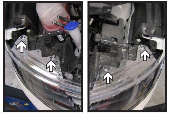
2. Using a T25 Torx, remove the four (4) screws from above the headlights. There are two (2) on each side.
