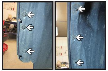
4. Using a 5.5MM socket, remove the six (6) bolts from the edge of the wheel well. Do this on both sides of the vehicle.
