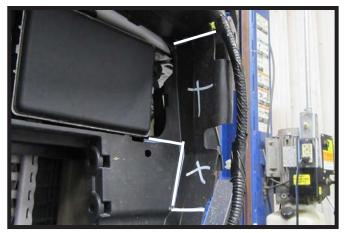
9. Using a utility knife remove the indicated areas on the driver side of the vehicle.
