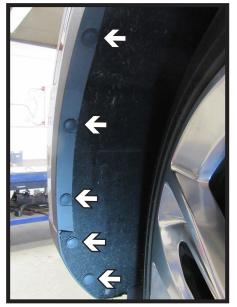
4. Remove the five (5) push pins from along the edge of the wheel well. Do this on both sides of the vehicle.
