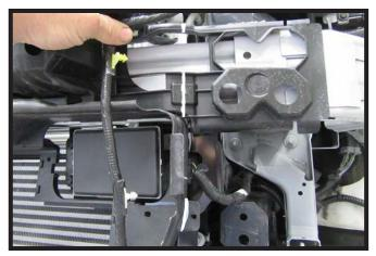
10. On the driver side of the vehicle remove the wiring harness from the push pin bracket. Using a utility knife remove the indicated areas.
