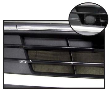
25. **Optional:** If there is an electrical plug for the engine block heater on the passenger side of the vehicle the following piece will need to be removed from the grill area as indicated.
