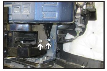
16. Using two (2) 3/8" bolts attach the Z bracket to the side plate as indicated.
