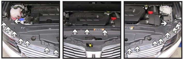
1. Remove the five (19) push pins from along the edge of the fascia. There are eight (8) on each side and three (3) in top middle. Remove top cover.
