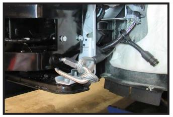
24. Attach the permanent baseplate safety cables to the provided convenience link on the baseplate. The photo above shows the recommended installation of the cables to frame of vehicle. Additional options may interfere with suggested mounting; in this case, secure the cables to a solid piece of the frame as described in the General Information sheet. Be sure the safety cables do not rub against any hoses or moving parts. Do this on **BOTH** sides of the vehicle.
