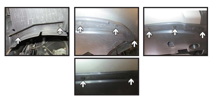
6. Using a 5.5MM socket, remove the eighteen (18) screws from the underside of the fascia. There are eight (8) on each side and two (2) in the center.
