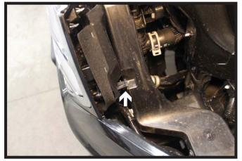
7a. Unsnap the fascia by the headlight locations. Pull the corners of the fascia away from the vehicle disconnecting any electrical connections and set the fascia aside.
