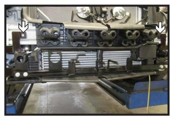
21. Using a 1/2" drill bit drill out top two (2) holes one (1) on each side. Metal is extremely hard so may need to start with a 1/4" drill bit then work up to a 3/8" drill bit and then eventually use a 1/2" drill bit to create the holes. Make sure to drill slowly.
