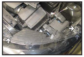
3. Using a 10MM socket remove the two (2) bolts (white) and one (1) push pin (gray) from the top of the headlight. Disconnect all electrical connections and set headlight aside. Do this on both sides of the vehicle.
