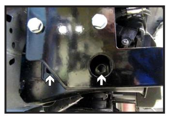
17. Using a 3/8" drill bit, drill out the bottom two (2) holes using the holes on the side plate as a guide. Install the provided 3/8" hardware. Do this on both sides of the vehicle.
