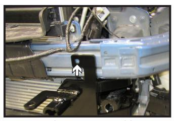
15. Using a 1/2" drill bit, drill one (1) hole as indicated on both sides of the vehicle.
