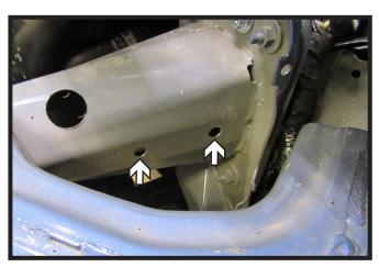
9. Using a 3/8" drill bit, ream out the two (2) existing holes. Do this on both sides of the vehicle.
