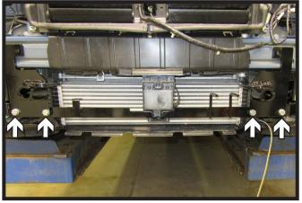
14. Install the cross-member on the back side of the side brackets with provided 1/2" hardware, making sure to not yet fully tighten the hardware. Then tighten the top two (2) bolts on both side plates followed by the bolts on the cross-member.
