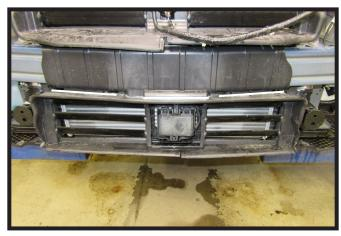
8. Using a 7MM wrench on backside (inset), remove the indicated bolt from the bottom of the shutter housing (left). Then using a utility knife cut along the top and around the edge of the housing as indicated (right). Unsnap the bottom of the shutter housing, remove, and set aside. It will not be reinstalled later.
