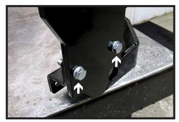
12. Attach the Z bracket to the back of each side plate using two (2) 3/8" bolts and hardware.
