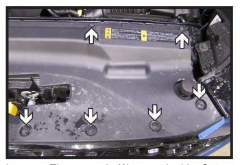
Remove the twelve (12) push pins from the fascia cover. There are six (6) on each side. Set cover aside to be reinstalled later.
