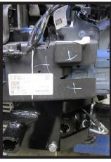
19. Using a utility knife, trim the bumper cover on both sides of the vehicle as indicated to allow clearance for the baseplate.
