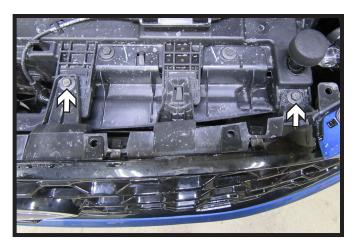
Using a 10MM socket, remove the four (4) bolts from the top edge of the fascia. There are two (2) on each side.
