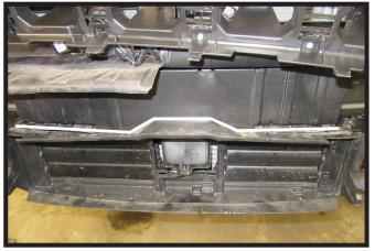
13. Unsnap the plastic piece above the shutter housing. Hold piece out of the way and mark the top of the shutter housing as indicated. Then cut shutter housing as indicate, remove shutters, and set aside. They will not be reinstalled later.
