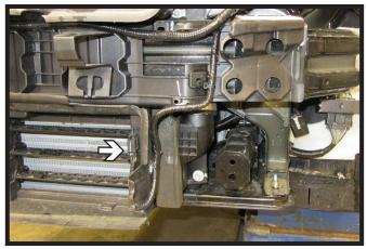
Unsnap the temperature sensor wire loom and place out of the way. It will be remounted later.
