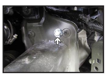
14. Using a 3/8" drill bit, drill one (1) hole as indicated on both sides of the vehicle then install the provided 3/8" hardware.
