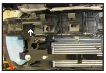
21. Using a 1/2" drill bit, drill one (1) hole as indicated on both sides of the vehicle.Note: May need to start with a smaller drill bit and work up to the 1/2" drill bit.
