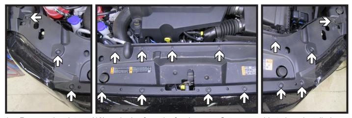
1. Remove the sixteen (16) push pins from the fascia cover. Set cover aside to be reinstalled later.
