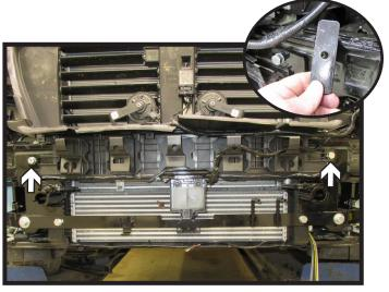
22. Install the 1/2" bolts with lock washer and a nut plate (inset) on the back side. Do this on both sides of the vehicle.
