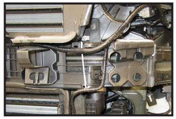
10. Using a reciprocating saw, trim the plastic piece as indicated. Do this on both sides of the vehicle.
