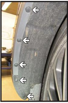
3. Remove the five (5) push pins from the edge of the wheel well. Do this on both sides of the vehicle.
