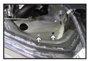
16. Using a 3/8" drill bit, ream out the two (2) existing holes on the side of the frame. Do this on both sides of the vehicle.
