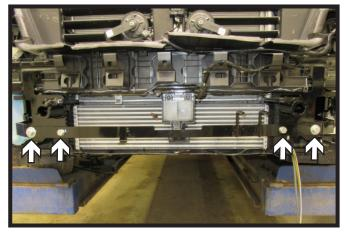
19. Install the cross-member on the front side of the side brackets with provided 1/2" hardware, making sure to not yet fully tighten the hardware. Then tighten the top two (2) bolts on both side plates followed by the bolts on the cross-member.
