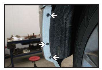
Using a 7MM socket, remove the three (3) screws from the edge of the wheel well.
