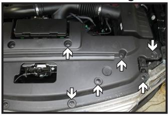
1. Using a Phillips screwdriver, remove the twelve (12) push pins from the top edge of the fascia cover. There are six (6) on each side. Set the cover aside.
