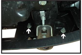
Using a 21MM socket, remove the two (2) nuts from the backside of the bumper. Do this on both sides of the vehicle.
