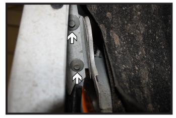
Using a 10MM socket, remove the two
