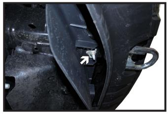
Using a 15MM socket, remove the nut in front of the lower valance. Do this on both sides of the vehicle.
