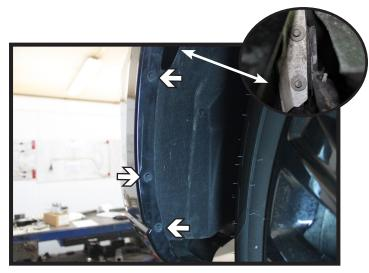
3. Using a 10MM socket, remove the three (3) screws from the edge of the wheel well. Along with the two (2) screws up inside the wheel well along the fascia joint. Do this on both sides of the vehicle.
