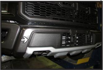
Unsnap the plastic cover from the face of the bumper. Do this on both sides of the vehicle.
