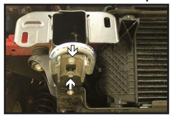
Using a 15MM socket, remove the two (2) bolts from the tow hook. Do this on both sides of the vehicle. Do not discard the existing hardware.
