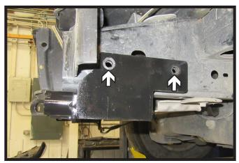
3. Using a 17/32" drill bit, drill the existing holes thru the frame. Install 1/2"-13 x 1-3/4" bolts with lock washers into the holes with 1/2"-13 nut plates on the inside of the frame. Do this on both sides of the vehicle. Fully tighten all hardware.
