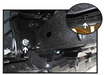
On the backside of the bumper, using a 21MM socket, remove the nut on the outside of the frame. Do this on both sides of the vehicle.
