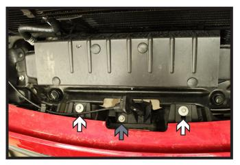
3. Unclip the cable from the clamp on the passenger side (left). Using a 8MM socket, remove the two (2) bolts from the middle of the bumper (right-white). Then using a 10MM socket, remove the center bolt from the middle of the bumper (right-gray). Remove the bumper from the vehicle disconnecting any electrical connections and set aside.
