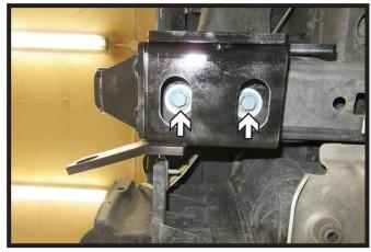
Install the baseplate to the frame with the existing hardware. Do this on both sides of the vehicle. Fully tighten all fasteners.
