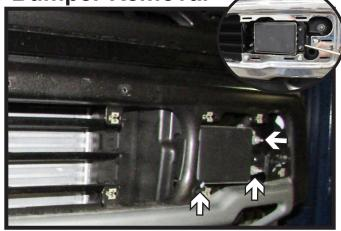
If equipped with Adaptive Cruise, using a 11MM socket, remove the three (3) nuts from the ACC sensor. Unsnap the sensor, disconnect the electrical connection and set aside.
