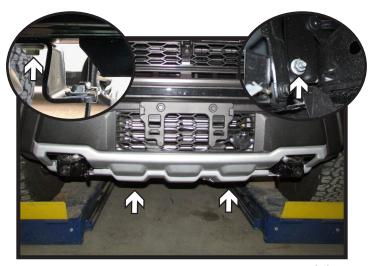
3. Using a 15MM socket remove the six (6) bolts holding the skid plate. Then using a 15MM socket remove the one (1) bolt from the skid plate bracket on each side of the vehicle (left inset).
