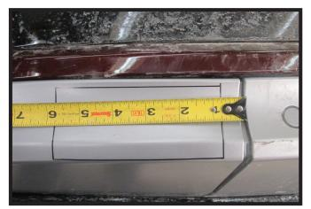
8a. Lincoln Navigator Models Only: Starting at 3/4" from the lip at the bottom of the fascia and 1/4" from the bumper. Draw a 5-1/2" wide by 2-1/4" tall rectangle as shown. Remove this area to allow room for the tab and convenience link. Do this on both sides of the vehicle.
