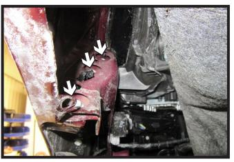
5. Pull the liner back, then using a 5.5MM socket remove the three (3) bolts. Do this on both sides of the vehicle.
