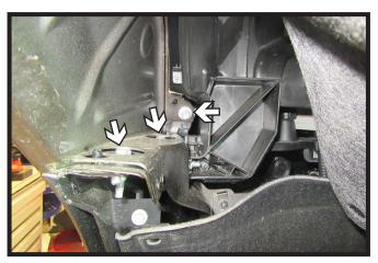
2. Pull the liner back, then using a 10MM socket remove the three (3) bolts. Do this on both sides of the vehicle.
