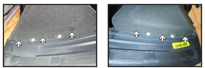
3. Using a 5.5MM socket, remove the six (6) bolts from the underside of the fascia in front of the tires.
