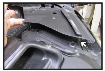
2. Before removing the fascia cover lift end and unsnap. Do this on both sides of the vehicle. Then remove fascia cover.
