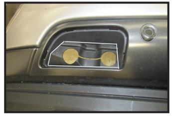
8b. Ford Expedition Models Only: Remove the area shown to allow room for the tab and convenience link. Do this on both sides of the vehicle.
