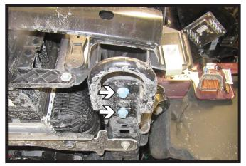
3. Using a 15MM socket, remove the two (2) bolts from the tow hooks. Do this on both sides of the vehicle.
