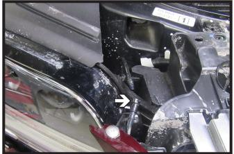
Lincoln Navigator Models Only: On the passenger side of the vehicle near the head light unhook the fluid line by squeezing and pulling apart.
