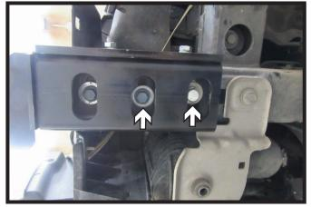
5. Make sure that the baseplate is tight against the frame of the vehicle and insert the back two (2) 1/2" bolts with flat washers and whiz nuts on the backside. Use Loctite<sup>®</sup> Red on these bolts. Once the back bolts are in place remove the front bolt and apply Loctite<sup>®</sup> Red and reinstall. Do this on both sides of the vehicle.
