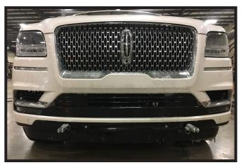
9a. Lincoln Navigator Models: Reinstall fascia and fascia cover. Reconnect fluid line on passenger side and electrical on driver side of the vehicle.
