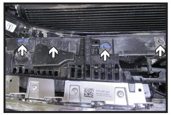
3. Using a 10MM socket, remove the four (4) bolts from the top of the fascia. Do this on both side of the vehicle.
