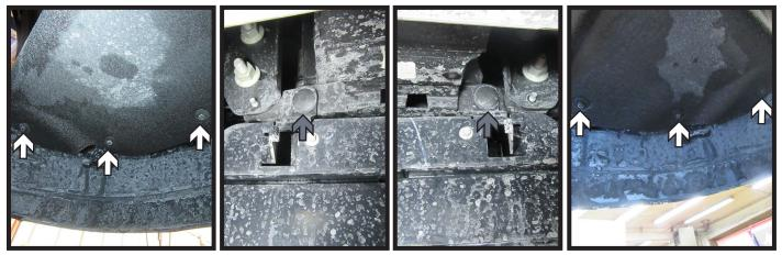
6. Using a 5.5MM socket, remove the six (6) bolts (white) and two (2) push pins (gray) from the underside of the fascia.
