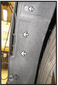
Using a 5.5MM socket remove the three
