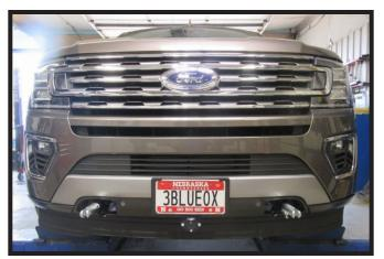
9b. Ford Expedition Models: Reinstall fascia and reconnect electrical on driver side of the vehicle.
