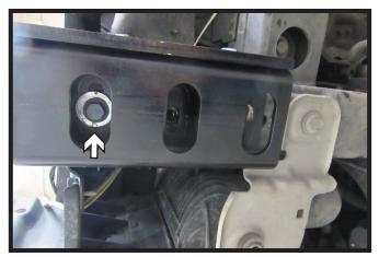
4. Slide the baseplate into place and hold. Start the first bottom 1/2" bolt with flat washer and whiz nut on backside. Do this on both sides of the vehicle. Do not use Loctite<sup>®</sup> Red at this time.
