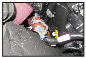
2. On the driver side of the vehicle unplug the indicated electrical. Then remove the front fascia.
