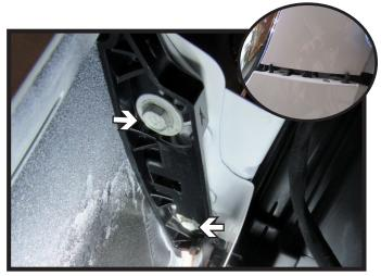
4. Pull back the wheel well liner and remove foam pieces. Using a 10MM socket, remove the two (2) bolts from the underside of the fascia joint. Pull fascia joint apart (inset). Do this on both sides of the vehicle.
