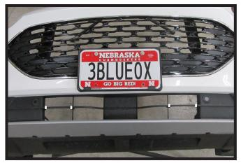
22. Remove the outer two (2) horizontal slats between the white marks as shown to allow room for the removable tabs and convenience links.
