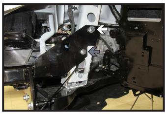
17. Insert nut plate through hole in the frame (left). Insert a 1/2" bolt with lock washer into the top hole (white) and a 3/8" bolt with lock washer into the bottom hole (gray). Do this on both sides of the vehicle.
