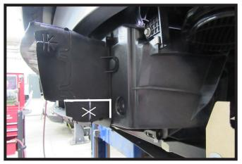
9. Using a utility knife, trim the plastic shroud as shown on both sides of the vehicle.
