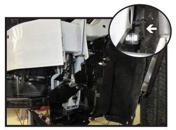
19. Reinstall the black box onto the driver side of the vehicle. Reattach the wire loom to the bottom bolt on the backside. If the box touches the baseplate bolt head, bend back plate slightly to create clearance (inset).
