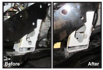
Using pliers, bend back the metal piece on the side of the frame creating an access hole for the nut plate. Do this on both sides of the vehicle.
