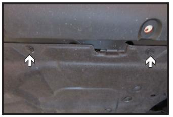
7. Using a 7MM socket, remove the four (4) bolts, two (2) on each side, from the underside of the fascia. Remove fascia and set aside to be reinstalled later.
