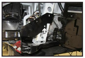
15. Using a 3/8" drill bit, drill out the bottom hole on the side of the frame using the baseplate as a guide. Do this on both sides of the vehicle.
