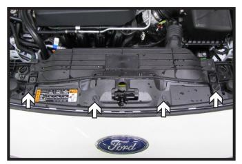
1. Using a 10MM socket, remove the four (4) bolts, two (2) on each side, from the top of the fascia.
