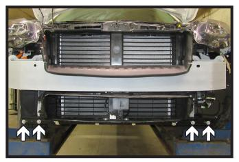
8. Using a 13MM socket, remove the four (4) bolts, two (2) from each side. Set aside to be reinstalled later.
