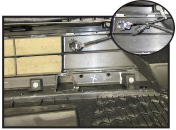
20. Unsnap temperature sensor from the back of the fascia (left). Cut plastic piece from the back of the fascia as shown (right). Zip tie the temperature sensor to the wire loom slightly above previous position (inset).
