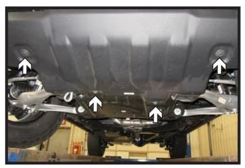
Using a 15MM socket, remove the four
