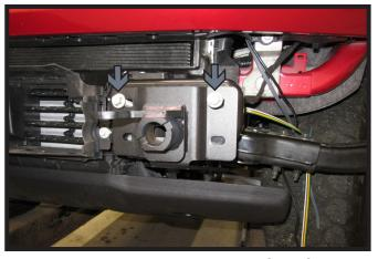
7. Start the one (1) 1/2" bolt (white) with flat washer and lock washer on the inside of the frame. Then on the front of the baseplate, start the top two (2) existing bolts (gray). Once the existing bolts have been started, fully tighten the two (2) side bolts. Remove the two (2) existing bolts. Do this on both sides of the vehicle.
