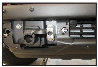
12. **Optional:** Using a 1/4" drill bit drill a hole in the bumper on the passenger side of the vehicle as shown. Bend breakaway bracket and install using a 1/4" x 1" bolt with flat washer and nylon lock nut.
