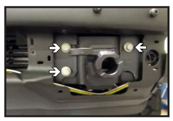
Reinstall bumper and install the three (3) existing bolts into the tow hook bracket/ baseplate holes. Do this on both sides of the vehicle.
