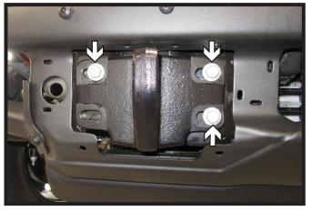
Using a 15MM socket, remove the three
