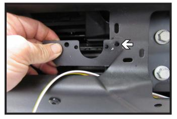
11. Hold electrical bracket up to the bumper on the driver side of the baseplate and mark spot. Using a 1/4" drill bit, drill a hole in the bumper. Attach bracket to the bumper using 1/4" x 1" bolt with flat washer and nylon lock nut.
