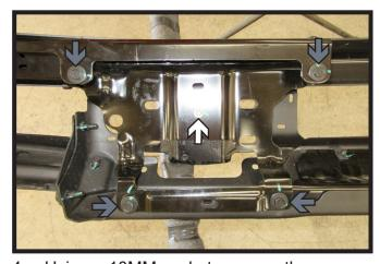
4. Using a 10MM socket, remove the one (1) bolt (white) from the tow hook bracket. Remove tow hook, it will not be reinstalled. Then using a 13MM socket, remove the four (4) bolts (gray) holding the tow hook bracket onto the bumper. Set bracket aside to be reinstalled on the bumper later. Do this on both sides of the vehicle.
