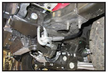
9. Attach the permanent baseplate safety cables to the provided convenience link on the baseplate. The photo above shows the recommended installation of the cables to frame of vehicle. Additional options may interfere with suggested mounting; in this case, secure the cables to a solid piece of the frame as described in the General Information sheet. Be sure the safety cables do not rub against any hoses or moving parts. Do this on BOTH sides of the vehicle. Reinstall belly pan.
