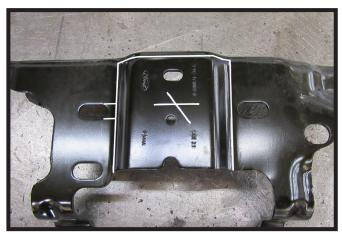
5. Using a reciprocating saw, cut and remove the indicated area of the tow hook bracket. Then slot the top hole as shown on the side of the bracket with two holes. Do this on both tow hook brackets. Reinstall brackets onto the bumper.
