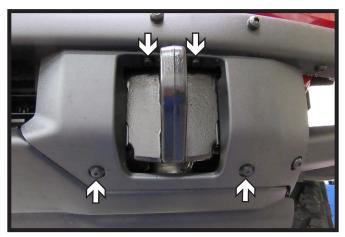
Remove the four (4) push pins from plastic tow hook cover. Unsnap cover and remove. Set cover aside to be reinstalled later. Do this on both sides of the vehicle.
