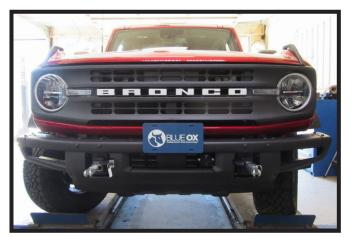
13. Hold the tow hook cover as close to its original position, mark and trim the covers around the convenience links and attachment tabs. Reinstall the covers.
