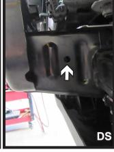
3. Using a 1/2" drill bit, drill out hole on the out side of the frame. Do this on both sides of the vehicle.
