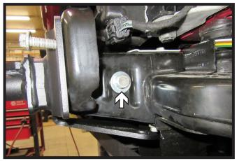
6. Slide the baseplate into the frame and start the one (1) 1/2" bolt with flat washer and lock washer on the outside of the frame. Do this on both sides of the vehicle. Do not fully tighten at this time.
