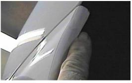
3. Using the phillips screw driver remove screw from each side of fascia corner. Remove four push pins just forward of front tire and four from the top side of fascia opening.
