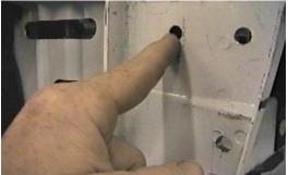
**4.** Drill out existing hole with the 13/32 drill bit.
