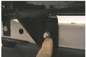
Using the baseplate as a template drill a 13/ 32" hole into cross member for lower supports. Insert items 4 and 7 into drill hole. Then insert item 2 into 1 1/4" hole to align with item 4 according to drawing on last page. Be sure and use loctite on all bolts before tightening.
