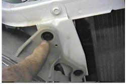
1. Remove three metric bolts from head light assembly with 10MM socket, pull forward, unplug, and set aside on both sides.
