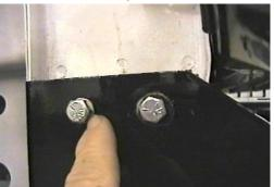
5. Hold baseplate and spacer plate to align with this drilled hole, insert items 5 and 7. Align item 2 with item 5 from inside frame end, both sides, do not tighten.
