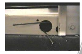
5. With the 1 1/4 inch hole saw cut a hole in the cross member front to gain access to interior.
