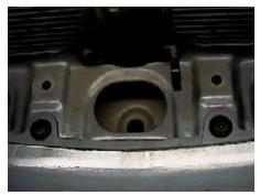
**4.** Just under plastic, in step three, are six phillips push pins to remove.
