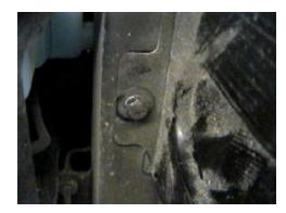
**10.** Remove six metric bolts on forward belly pan using the 12MM socket and set aside.
