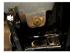
6. Remove two phillips screws from the bottom middle of fascia.
