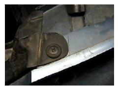
**3.** Just under headlight assembly are phillips push pins to remove, both sides. Lift vertical black plastic, remove plastic over the top of metal bumper and set aside.
