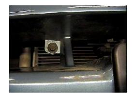
**8.** Using the 10MM socket, remove two metric bolts in fascia opening.
