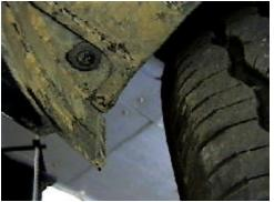
7. Just forward of front tire are two phillips push pins to remove, both sides.
