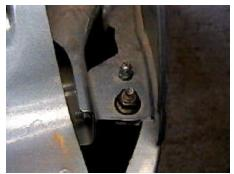
**5.** Remove one metric bolt just behind head light assembly using the 7MM socket, both sides.
