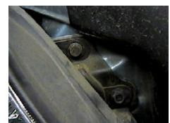
2. Remove three metric bolts from headlight assembly with the 10MM socket, pull forward, unplug electrical and set aside, both sides.
