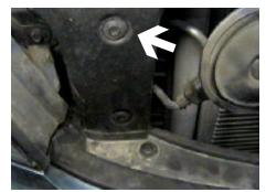
**1.** Remove the two phillips push pins from black plastic on both sides. remove six phillips push pins on plastic covering metal bumper.
