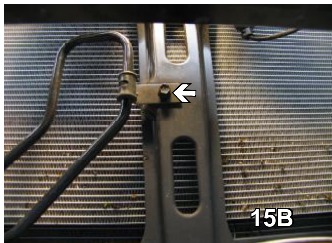
15. On the passenger side, using a 10MM socket, remove the three bolts holding the transmission fluid line. Let the line swing down during installation of the baseplate. Set bolts aside for later reinstallation.
