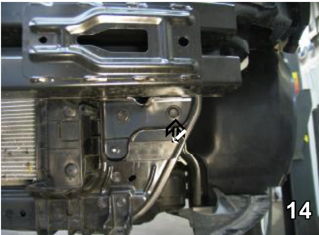
14. Using a 12MM socket, remove the bumper bolt. Do this on both sides.
