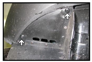
3. Remove the two (2) push pins from the underside outer edge of the fascia. Do this on both sides of the vehicle.
