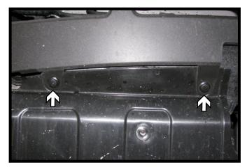
4. Remove the two (2) push pins from the underside inner edge of the fascia. Do this on both sides of the vehicle. Pull the outer top edges of the fascia outwards and pull fascia forward to remove from the vehicle.
