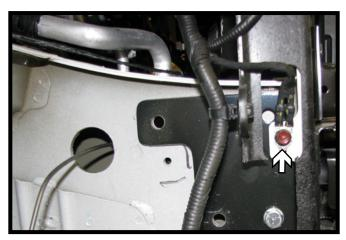
9. Insert a 3/8"-16 x 1-1/4" bolt with lock washer into the front hole and secure with a 3/8"-16 nut plate. Re-level the baseplate and tighten the 3/8" hardware. Temporarily remove the ground strap, and drill the remaining baseplate holes with a 13/32" drill bit. Do this on both sides of the vehicle.
