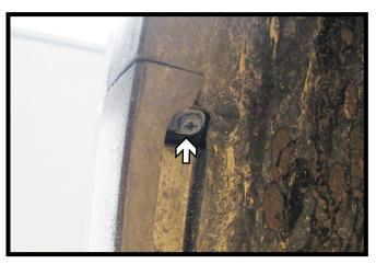
Using a 8MM socket, remove the screw from the top edge of the wheel well. Do this on both sides of the vehicle.
