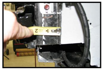
6. On the side of the frame measure over 1-1/2" from the edge and trim the corner of the plate off as shown using a reciprocating saw. Do this on both sides of the vehicle.
