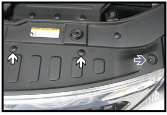
Using a 10MM socket, remove the screw from the top outer edge of the fascia (gray). Then remove the two (2) push pins (white). Do this on both sides of the vehicle.
