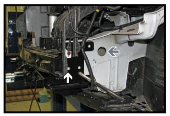
8. Clamp the baseplate into position as close to level as possible as shown.
