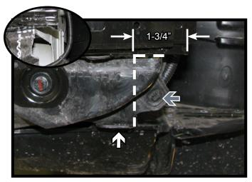
5. Remove the push pin from underneath the bumper attaching the plastic guard. Unsnap the wiring loom from the bracket (gray). Measure over approximately 1-3/4" from edge of the bumper and cut the corner off flush with frame using a reciprocating saw. Do this on both sides of the vehicle.
