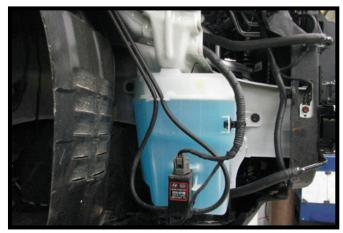
7. Disconnect the electrical connections and fluid lines from the washer reservoir. Using a 10MM socket, remove the reservoir bolts and set the washer reservoir aside.
