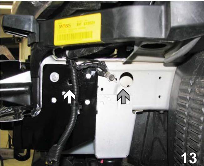
13. Using a 13/32" drill bit with the base plate as a template drill one hole (white arrow). Using a 1 1/4" hole saw, drill a hole in the frame next to the ground wires for the nut plates (gray arrow). Do this on both sides of the vehicle. Be sure to install only one bolt assembly per side to stabilize baseplate before drilling the remaining holes.
