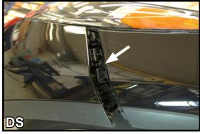
4. Firmly lift up on the sides. If necessary, a flat screwdriver may be used. We recommend you place a cloth over the screwdriver to prevent scratching your vehicle surface.
