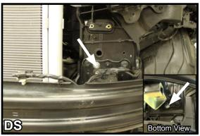
11. For additional support when reinstalling the front bumper you will need to drill two (2) 3/8" holes into the bumper mounting plate. Once the bumper is reinstalled securely, reattach the temperature sensor.
