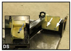
10. With the bumper lying upside down, place the baseplate on top and align the outer most holes. Using a 13/32" drill bit, drill the inner hole and the top hole.
