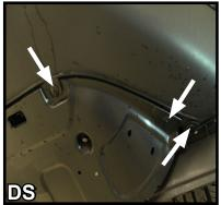
3. Remove the three (3) push pins that are located underneath the vehicle towards the outer edge. There are two (2) push pins located in the center of the vehicle that also need to be removed.
