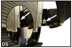
6. After removing the plastic brackets trim the aluminum clips.
