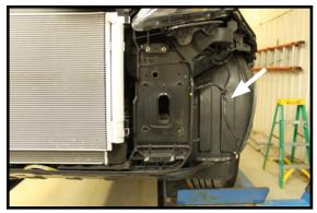
The temperature sensor will need to be temporarily relocated. Unclip it from the bumper and move off to the side.
