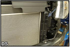
5. Remove the plastic brackets along side the radiator by sliding upward.
