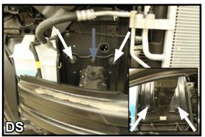
8. To remove the front bumper, use a 12MM socket to remove the four (4) outside bolts on the bumper mount bracket. There are two (2) on the top and two (2) on the bottom. The one (1) center bolt on top requires a 10MM socket.
