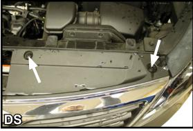
1. With a 10MM socket, remove the bolt from the top portion of the fascia on each side. Remove push pin, one (1) per side.
