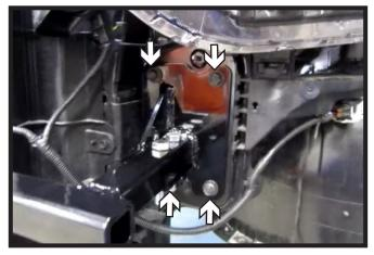
11. Install the four (4) existing 8MM bolts. Add hardware to the two (2) 1/2" bolts on the baseplate. Tighten all bolts at this time. Do this on both sides of the vehicle.
