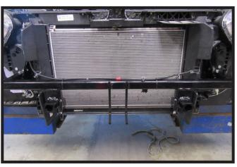
13. Zip tie the temperature sensor and wire loom to the top of the baseplate using the provided zip ties.
