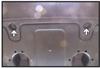
3. Remove the ten (10) push pins from the underside of the fascia, four (4) on each side and two (2) in the middle. Remove fascia and set aside to be reinstalled later.
