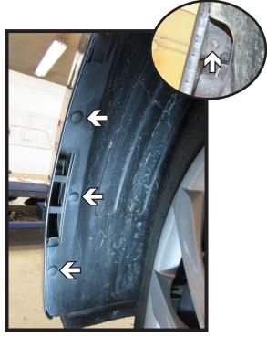
2. Remove the three (3) push pins from along the edge of the wheel well. Then using a 8MM socket remove the one (1) bolt (inset). Do this on both sides of the vehicle.
