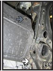
5. Using a 10MM socket, remove the two (2) bots from the passenger side and one (1) bolt from the driver side (white) of the belly pan. Then remove the one (1) push pin from each side of the belly pan (gray). Remove belly pan and set aside to be reinstalled later.
