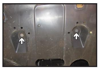
Using a 10MM socket, remove the four (4) bolts, two (2) on each side from the front portion of the belly pan.
