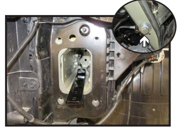
9. Insert frame support bracket as shown. Start the one (1) 5/8" bolt from the bottom of the frame with hardware (inset). Do this on both side of the vehicle.
