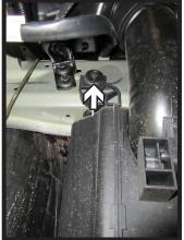
6. Using a 10MM socket, remove the three (3) bolts from the air baffle on the driver side of the vehicle. There are two (2) on the outside of the frame and one (1) on the backside. Remove baffle and set aside to be reinstalled later.
