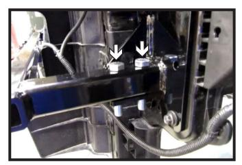
10. Slide the baseplate into place. Insert the two (2) 1/2" bolts without hardware into the baseplate lining up the baseplate and support bracket holes. Do this on both sides of the vehicle.
