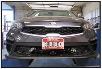
15. Reinstall air baffle. Hold the fascia as close to its original position, mark and trim the fascia around the convenience links and attachment tabs. Reinstall the belly pan and fascia.
