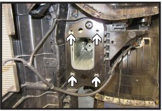
7. Using a 12MM socket, remove the eight (8) bolts, four (4) on each side, from the bumper. Unsnap wire loom and temperature sensor from the bumper, they will be repositioned later. Remove bumper and set aside, it will not be reinstalled later.
