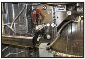
12. Using a 3/8" drill bit, drill the one (1) hole as indicated. Install the 3/8" bolt with hardware. Do this on both sides of the vehicle.
