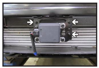
Using a 10MM socket, remove the three
