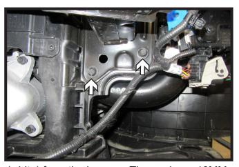
6. Using a 12MM socket, remove the four (4) bolts (white) from the bumper. Then using a 10MM socket, remove the one (1) bolt (gray) from the bumper. This bolt is above the bumper on the driver side and below the bottom of the bumper on the passenger side. Do this on both sides of the vehicle. Remove bumper and set aside, it will not be reinstalled.
