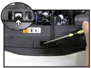
Using a flat screw driver, pop out the plastic piece in the middle of the fascia cover. Using a 10MM socket, remove the one (1) bolt (inset)
