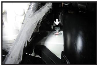
11. Start the two (2) 1/2" bolts with hardware, one (1) on each side, on the inside of the frame as shown. On the driver side this can be accessed from the underside of the vehicle and from above on the passenger side. When installing the bolt on the passenger side, it is easier to do this from the underside of the vehicle. Leave loose at this time.
