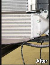
9. Using a reciprocating saw, trim the shroud on each side so that the bottom is flush and the sides are removed as shown.
