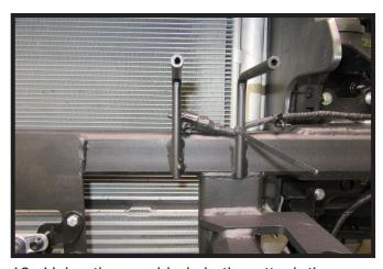
16. Using the provided zip ties attach the temperature sensor loom to the baseplate on the driver side of the vehicle as shown.
