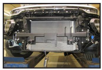
13. Start the remaining four (4) bolts, two (2) on each side to the front of the baseplate. Set the cross tube onto the side brackets. Place the four (4) 1/2" bolts with flat washer and lock washer into holes. Do not add hardware to the bottom of bolts.
