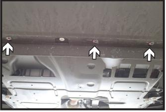
Across the center on the underside of the vehicle, use a T30 Torx to remove three (3) screws. *DO NOT* remove the silver screw.
