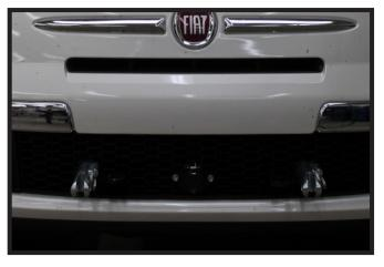
11. Hold the fascia as close to its original position, mark and trim the fascia around the convenience links and attachment tabs. Reinstall the fascia.
