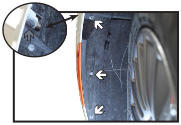
2. In the wheel well, using a Phillips screwdriver, remove the three (3) screws (white). In upper corner of the wheel well, using a T30 Torx, remove the one (1) screw (gray). Do this to both sides of the vehicle.
