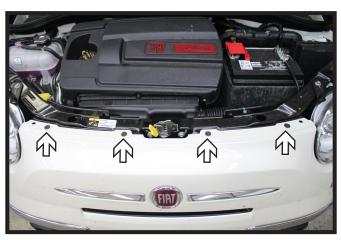
1. Using a T30 Torx, remove the four (4) screws from the top edge of the fascia.
