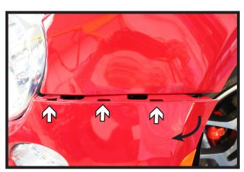
Unclip the fascia on the side. Once the fascia has been released, unplug all electrical connections. Next, firmly pull the fascia outward to remove. Set the fascia aside.
