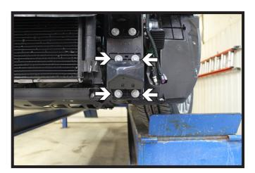
7. Using a 14MM socket, remove the four (4) lower bolts in the bumper horn bracket. Do this on both sides of the vehicle. These brackets will NOT be reinstalled.
