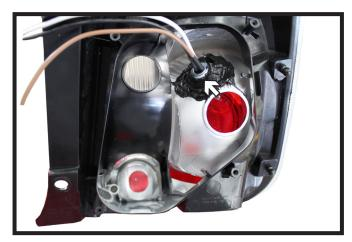
12. Possible location for BX8869 wiring kit: On the side of the tail light, using a T20 Torx remove the four (4) screws. Remove the back piece. Using a 1/2" drill bit, drill a hole in the plastic piece. Put the wires through the hole and silicon around it. Do this on both sides.
