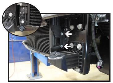
6. Remove the air deflector, use a 8MM socket to remove the two (2) screws on the driver side (white) and the one (1) screw on the passenger's side (gray). The deflector will NOT be reinstalled.
