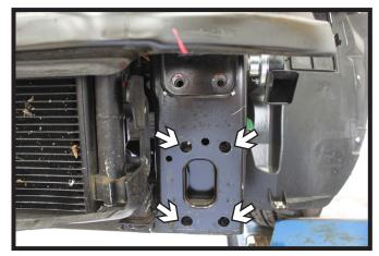
8. Align the baseplate with the four (4) holes and use the existing bolts to secure the baseplate. Do this on both sides of the vehicle.
