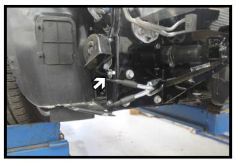
9. On the passenger side, reinstall the horn to the existing stud.
