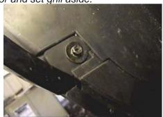
Just forward of front tires, in wheel well, is one metric bolt to remove using either the phillips screw driver or a 7MM socket, both sides.
