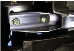
7. Remove the four metric nuts from cross tube, just below metal bumper, with the 16MM socket and two metric bolts from the center braces with the 10MM socket, set tubing aside. Tubing will not be reinstalled. Also remove the two metric nuts just above the metric nuts on cross tube seen in the photo, both sides. Some 2005 Models may not have this cross tube to remove.
