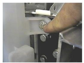
7. Reinstall washer reservoir using back existing metric bolt and nut. Then install the 6MM x 30MM bolt in the front holes. Be sure all water and all electrical lines are plugged in properly.
