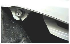
**3.** Just forward of front tire, on fascia's corner, remove one metric bolt using the 10MM socket. Pull fascia forward and unplug electrical connections. Some models may have headlight washer system. If needed, disconnect water lines. Set fascia aside.
