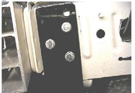
Using the baseplate as a template, drill remaining holes with the 13/32" drill bit. Insert nut plate into 1 1/4" hole to align with the drilled holes, install 3/8" bolt and lock washer. Tighten all bolts. Be sure to use loctite on all bolts before tightening. Tighten all bolts according to torque chart in General Instruction Sheet.
