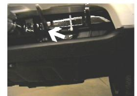
**9.** It may be necessary to trim the back edge of first vertical style on both side with the utility knife.
