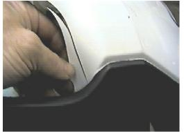
8. Hold fascia in place on vehicle, mark and trim areas on the back edge of fascia opening on both sides, see photo.
