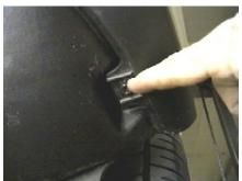
2. Remove six metric bolts from the bottom edge of front fascia using the 10MM socket.
