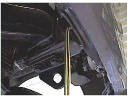
1. Using the 17MM socket, remove the metric bolts from driver's side tie down bracket. Tie down bracket will not be reinstalled.
