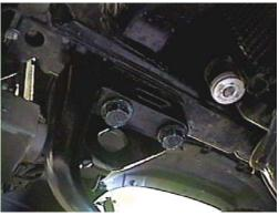
2. Using the 17MM socket, remove two metric bolts from tow hook/ tie down bracket, on passenger's side. Tie down bracket will not be reinstalled.
