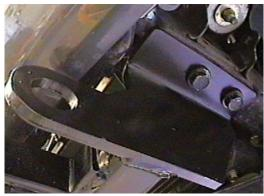
3. Hold baseplate to align with holes of tie down bracket on driver's side and fasten existing bolts, do not tighten. Be sure and use loctite on all bolts before tightening.
