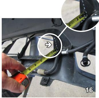
16. On the edge of the fascia opening, trim an inch in and taper back to the corner as shown. Do this on both sides.
