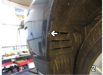
2. Using a 25 TORX, remove the bolt just forward 3. Just forward the front tire, above and inside the front tire. Do this to both sides and set aside for later reinstallation.
