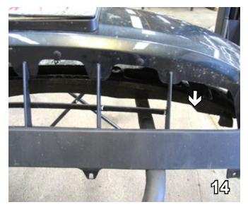
14. Trim the fascia. Remove the two outside horizontal styles, using a utility knife. One is shown, do the same on the other side.
