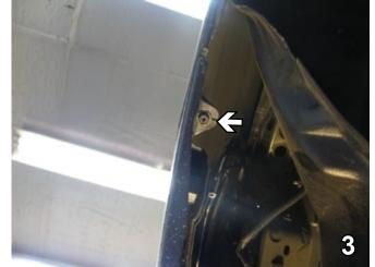
wheel well cover, use a 10MM socket to remove the screw. Set screw aside to be reinstalled later. Do this to both sides of the vehicle.
