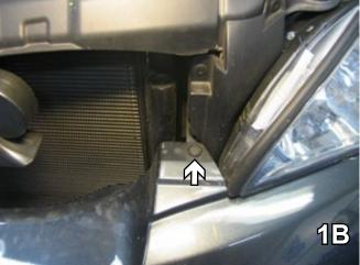
1. Remove the fascia by removing 3 pushpins with a flat screwdriver. The first one is on the middle (1A) and one is just inside of headlight (1B). Do this on both sides. Set push pins aside to be reinstalled later.
