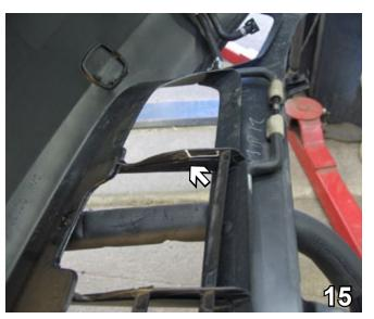
15. On the back side of the fascia, trim the two outside vertical styles as needed. (Hold fascia in place and trim as needed.) Do this to both sides.
