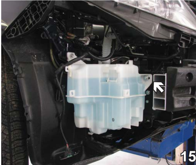
15. Reinstall washer reservoir. Do not use the existing bolt in the area shown, use a 6MM -1.0 x 30MM hex bolt with 1/4" lock washer, 1/4" flat washer and 1/2" spacer. Connect the hoses and plug in electrical connections.
