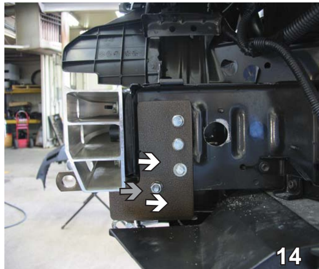
14. In the lowest hole (grey arrow), use a 3/8-16 x 1 1/4" hex bolt with a 3/8" lock washer and 3/8-16 hex nut. Note: The lower bolt is inserted from the back side of frame webbing (see page 2). The other bolts are 3/8-16 x 1 1/2", attached to 3/8 lock washer and 3/8-16 nut plates. Also cover the hole on the back. Do this to both sides.
