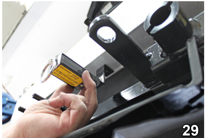
29. Optional: Mount the breakaway bracket to the bottom of the metal bumper, all the way back to the bottom ridge of the bumper. Position it half-way between the electrical rods and the convenience link. Install using 1/4-20 x 3/4 hex bolt, 1/4-20 hex nyl nut, and #10-16 x 1" self-drilling screw.
