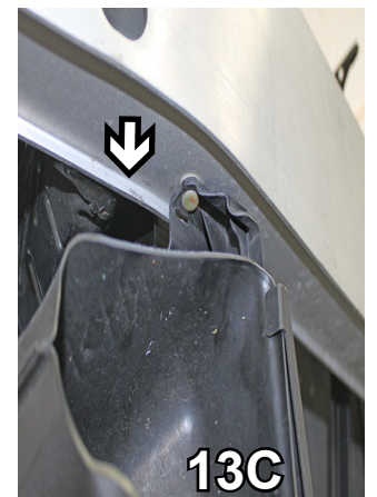
13. To remove the air baffles, with a 10MM socket, in front of the tire, remove bolt (13A), under the air baffle, remove 2 bolts (13B) and unhook the air baffle at the bottom of the metal bumper (13C). Do this on both sides. Pull down air baffles to remove and set aside air baffles and bolts to be reinstalled later.
