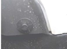
**5.** Remove six push pins from the bottom edge of the fascia. Pull fascia forward and set aside.
