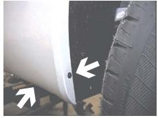
4. Forward of front tires are two metric bolts in wheel well and two metric bolts on the lower edge of fascia to remove with the 7MM socket, both sides.
