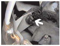
1. Remove wing nut on top side of head light assembly, pull assembly forward, unplug and set aside, both sides.
