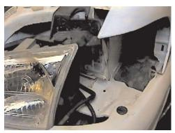
2. Remove one push pin from under head light assembly, both sides.
