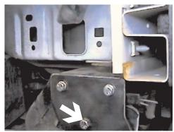
9. Using the baseplate as a template, drill lower hole with the 13/32" drill bit, both sides. Align 1/2" spacer plate between lower hole on end plate and drilled hole in tie down bracket on passenger's side. Insert 3/8" hex bolts into lower hole on passenger's side, tighten lock washer and hex nut on back side of tie down bracket. Be sure and use loctite on all bolts before tightening. Torque all bolts according to torque chart in General Instructions.
