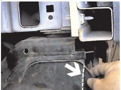
7. Using the reciprocating saw, cut 1 3/4"- 2" off of passenger's side tie down bracket to open area for baseplate (Vehicles may vary).
