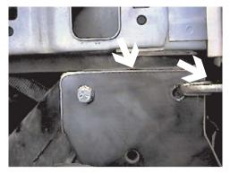
8. Align baseplate to the top, front edge of lower frame support, clamp with the vise grips on both sides. Using the baseplate as a template, drill the top two holes with the 13/32" drill bit, both sides. Insert nut plate into end of frame to align with drilled holes and tighten 3/8" hex nut and lock washer as shown in drawing on page 3.
