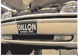
6. Remove two push pins from top edge of lower fascia opening, between fog lights. Pull fascia forward and set aside.
