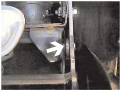
10. Insert spacer washers between lower hole on end plate and drilled hole in tie down bracket on driver's side. Some vehicles may only need one spacer to fill gap. Insert 3/8" hex bolts into lower hole on driver's side, tighten lock washer and hex nut on back side of tie down bracket. Be sure and use loctite on all bolts before tightening. Torque all bolts according to torque chart in General Instructions.
