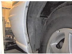
3. Just forward of front tires are two phillips screws to remove, both sides.
