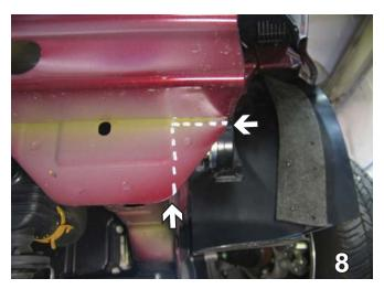
8. Using a reciprocating saw, trim on the front of the frame under the bumper, as indicated in the photo. Do this to both sides.
