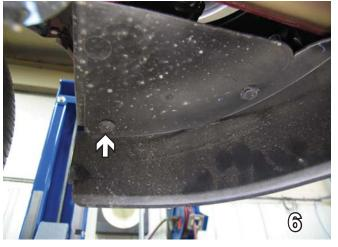
Underneath the fascia, use a flat screw driver to remove two push pins. Do this to both sides of the vehicle. Set the push pins aside to be reinstalled later.
