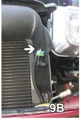
9. The sensor in 9A needs to be moved up to a 1/4" drilled hole shown in 9B.
