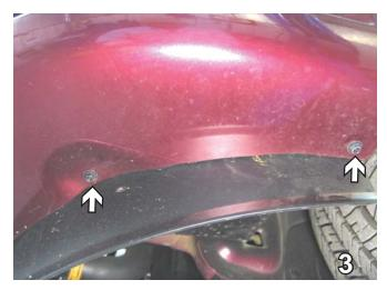
Using a 7MM socket, remove two bolts from the lower edge of the fascia. Do this to both sides of the vehicle. Set bolts aside to be reinstalled later.
