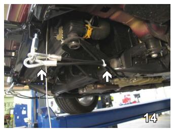
14. Install the baseplate safety cables to the frame of the vehicle. If the vehicle has additional options which interfere with mounting the permanent baseplate safety cables, secure the cables to a solid piece of the vehicle frame as described in the instructions included with the permanent baseplate safety cables. Be sure the safety cables do not rub against any hoses or moving parts.
