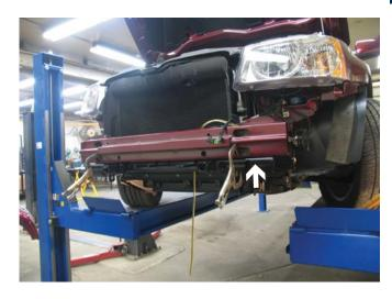
Slide the baseplate up, as far forward as possible and clamp to the bottom of the bumper.
