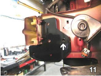
11. Using the baseplate as a template, with the 13/32" drill bit, drill one hole. Tighten with 3/8-16 x 2" bolt, 3/8" lock washer and 3/8-16 nut plate inserted into the frame. Use loctite. Do this on both sides. Drill the remaining holes.
