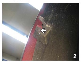
Just forward of the front tire, move the wheel well cover, use a 7MM socket to remove the bolt. Do this on both sides and set aside for later reinstallation.
