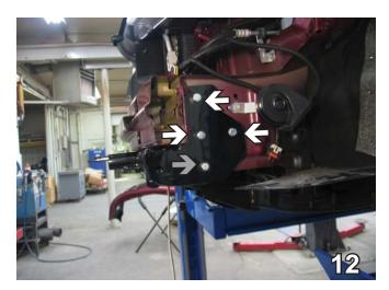
12. Insert into the top three holes (white arrows), 3/8-16 x 2" bolts with Loctite, 3/8" lock washers and attach to 3/8-16 nut plates inserted into the frame (figure 13A) and tighten. Insert into the bottom hole (gray arrow), 3/8-16 x 1 1/2" bolt with Loctite, 3/8" lock washer and attach to 3/8-16 nylon nut on the back (figure 13B). Do this on both sides.
