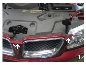
Remove three push pins from the flat plastic piece on top. Set push pins aside to be reinstalled later.
