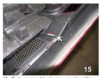
15. On the inside of the fascia, using the utility knife cut off the tab as shown. Do this on both sides.
