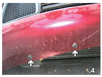
Using a flat screw driver, remove five push pins from the lower edge of fascia all the way around. Set push pins aside to be reinstalled later.
