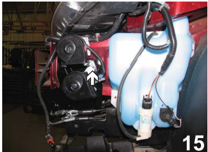
15. Reinstall the horn on the driver's side with a 6MM x 30MM bolt and 5/16" flat washer.
