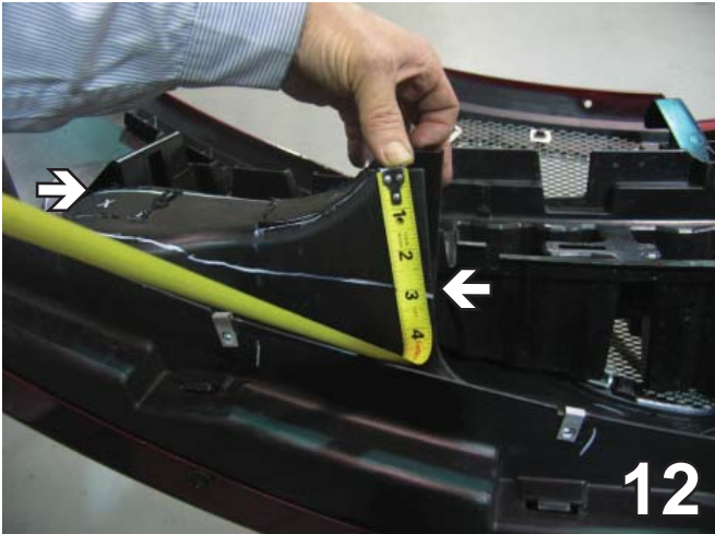
12. Mark the side of the air dam straight down 3 inches where the hole is and around the contour of the air dam mold around the outside edge. Remove the plastic piece. Do this on both sides.
