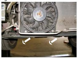
Using the 10MM socket, remove the two metric bolts from the lower fan assembly, pull fan assembly down to remove from radiator and set aside.
