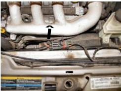
7. Pull electrical coupler on top of radiator toward driver's side to release from bracket and unplug.
