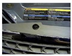
**1.** Remove the three push pins from the top side of grill, set grill aside.
