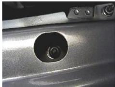
**5.** Using the 13MM socket, remove six metric bolts from metal bumper, pull forward and set aside. **NOTICE:** Pull air baffle tube straight down on passenger's side to release and expose inner frame area, set tube aside.
