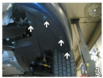
Remove four pushpins from the bottom edge of the fascia, just forward of the front tire. Set the pushpins aside to be reinstalled later. Do this to both sides of the vehicle. Pull fascia's upper corners out to the side of the vehicle and straight forward. Set the fascia aside carefully to be reinstalled later.
