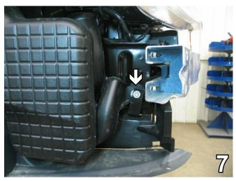
Using a 10MM socket, remove one metric bolt from the air baffle on the passenger's side. Set the bolt aside to be reinstalled later.
