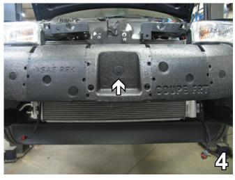
4. Remove one pushpin from the styrofoam bumper. Set styrofoam bumper and pushpin aside to be reinstalled later.
