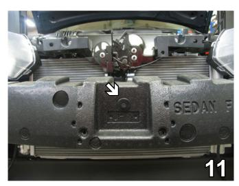
11. Reinstall the horn bracket on the driver's side. Reinstall the metal bumper and styrofoam to their original positions.
