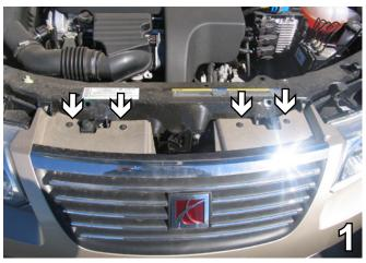
Using a 7MM socket, remove four metric bolts from the top side of the fascia. Set the bolts aside to be reinstalled later.
