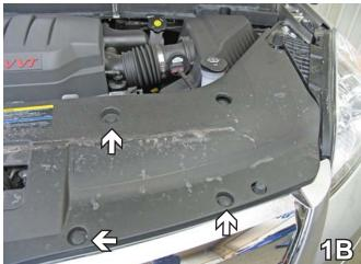
Using a flat screwdriver, remove 4 push pins from the flat plastic piece on top. Do this to both sides of the vehicle. Set push pins aside to be reinstalled later.
