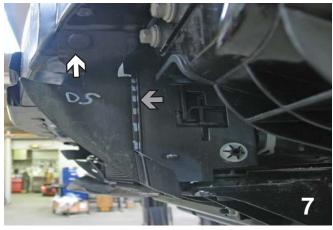
7. Using a flat screwdriver, remove pushpin (see white arrow) and then using a utility knife, cut along dashed line shown in the photo above (see grey arrow). The plastic piece will not be reinstalled and can be discarded. Do this to both sides of the vehicle.
