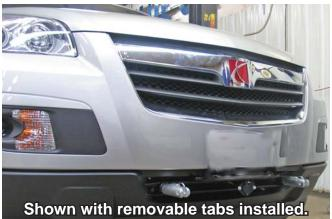
If the baseplate is in an accident, it must be replaced. DO NOT use it again! An accident can cause unseen damage and using it again could result in more damage or serious injury. DO NOT use the paseplate if it is damaged or missing parts.
