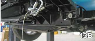
13. Attach permanent baseplate safety cables to the convenience link on the baseplate (see photo 12A). Photo 12B shows recommended installation of the cables to frame of vehicle. If vehicle has additional options (not shown above) which interfere with mounting permanent baseplate safety cables, secure the cables to a solid piece of the vehicle frame as described in instructions included with the permanent baseplate safety cables.
