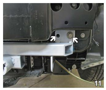
11. Slide baseplate up, so it matches up with the existing holes of the bumper. Insert the existing bolts from the bumper and tighten them down with a 15MM socket so they are snug. Do this to both sides of the vehicle.
