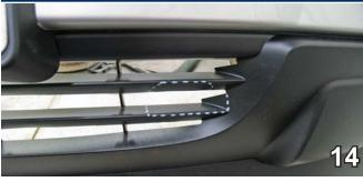
14. Align the fascia to its original position, and using a hack saw knife, trim out the opening in the grille for the attachment tabs, using the photo above as a template. Do this to both sides of the vehicle.
