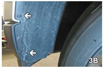
Using a phillips screwdriver, remove four phillips screws just forward of the front tire, on the wheel well. Set screws aside to be reinstalled later. Do this to both sides of the vehicle.
