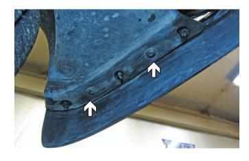
Using a phillips screwdriver, remove two screws from just forward of the front tire underneath. Set screws aside to be reinstalled later. Do this to both sides of the vehicle. 5
