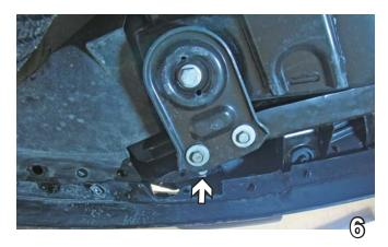
6. Using a 10MM socket, remove a bolt from the brace for the fog light. In the picture above, the bolt is hidden slightly (see white arrow). Set bolt aside to be reinstalled later. Do this to both sides of the vehicle. The fascia is then ready to be removed from the vehicle and carefully set aside to be reinstalled later.
