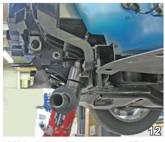
12. Using the baseplate as a template, drill the two bottom holes into the frame with a 17/32" drill bit. Insert the 1/2" nut plates into the frame and align with drilled holes. Insert a 1/2-13x1 1/2" hex bolt and 1/2" lock washer into each hole and tighten down with a 3/4" socket. Do this to both sides of the vehicle.
