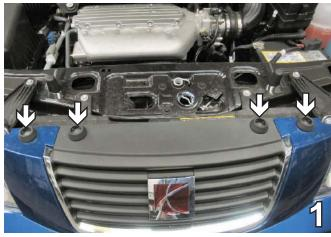
Remove four metric bolts with hood bumpers from the top side of the front fascia using a 7MM socket. Set aside to be reinstalled later.
