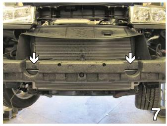
Remove two large push pins from the Styrofoam bumper. Set Styrofoam and push pins aside to be reinstalled later.
