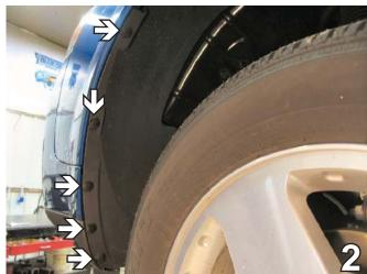
2. Just forward of the front tires, on the edge of the wheel well, remove five push pins. Set aside to be reinstalled later. This is done to both sides of the vehicle, the driver's side is shown.
