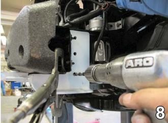
Slide the baseplate onto the outside of the frame rail just behind bumper bracket and up as far as possible. Clamp the baseplate to the end of the metal bumper on both sides of the vehicle. Using the baseplate as a template, drill three holes into the side of the frame rail with the 13/32" drill bit. Do this to both sides, the driver's side is shown.
