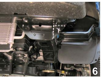
Using a reciprocating saw, make a horizontal cut just below the metal bumper on the bumper bracket into the outside edge of the frame. Do this on both sides of the vehicle. Make a vertical cut on the bumper bracket flush with the outside of the frame channel. Do this on both sides of the vehicle. BE sure NOT to cut into the frame channel with either of these cuts. This will open the area to prepare it for baseplate installation. The driver's side is shown.
