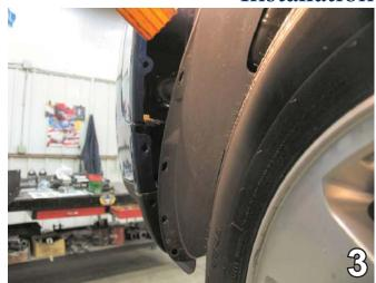
Pull wheel well cover back and remove one metric bolt from the fascia's corner using a 10MM socket. Set aside to be reinstalled later. This is done on both sides, the driver's side is shown.
