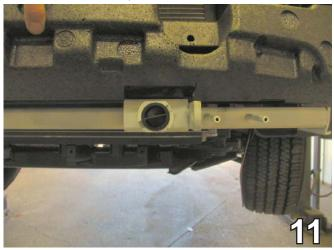
11. With baseplate installation completed, set Styrofoam as close to its original position as possible. Mark and cut the bottom of the Styrofoam 1/2" deep around the attachment tab receiver area with a utility knife and remove this portion of the Styrofoam. This is done to both sides of the vehicle, the driver's side is shown. Reinstall Styrofoam with the existing two large push pins.
