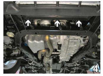
Remove three push pins from lower edge of fascia. just behind fascia's lower air dam. Set aside to be reinstalled later.
