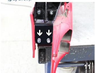
11. Again, using the baseplate as a template, drill the two side holes through the bumper on both sides using a 13/32" drill bit. Insert a 3/8-16 x 1 1/2" hex bolt with a 3/8" lock washer and a 1/4 x 1 x 1" nut plate. Tighten with Loctite Red. Do this on both sides of the vehicle.
