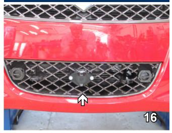
16. Reinstall the fascia, belly pan and all electrical connections using the existing bolts and push pins. Optional: Attach the electrical bracket to the center of the fascia (white arrow).
