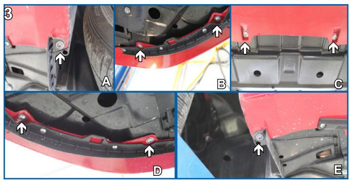
3. Starting in front of the driver's side wheel, on the underside of the fascia, use a Phillips screwdriver to remove eight total screws from the rim of the fascia. Set screws aside to be reinstalled later.
