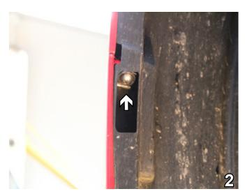
2. Use a Phillips screw driver and remove the screw concealed in the front of the wheel well. Do this on both sides of the vehicle. Set aside screws to be reinstalled later.
