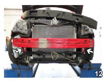
12. Reinstall the bumper to its original position by using eight 8MM -1.25 x 30MM hex bolts with 8MM lock washers and 8MM flat washers. Tighten with Loctite Red. Reintall the black styrofoam section of the bumper. Reinstall all electrical connections to the bumper.
