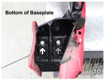
10. Using a 13/32" drill bit and the baseplate as a template, drill through the bottom back hole into the bumper (white arrow). Insert a 3/8-16 x 1 1/2" hex bolt with a 3/8" lock washer and a 1/4 x 1 x 1" nut plate. Do this on both sides first. Tighten with Loctite Red. Then repeat procedure on bottom front hole on both sides (gray arrow).
