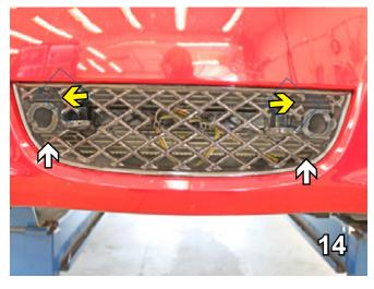
14. To allow for the attachment tabs, place the fascia into position and use a utility knife to trim the holes for the tabs (white arrows). Excess trimming is required to allow the fascia to fit over the hood latch for reinstallation (yellow arrows).
