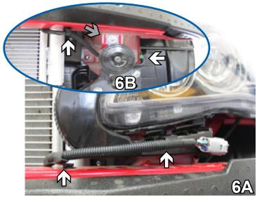
6. Disconnect the electrical cord from the front bumper, located in front of each headlight (6A), and below the front bumper (6B, white arrows). Use a 4MM socket and remove the bolt from the horn bracket (6B, gray arrow). Do this on both sides of the vehicle.
