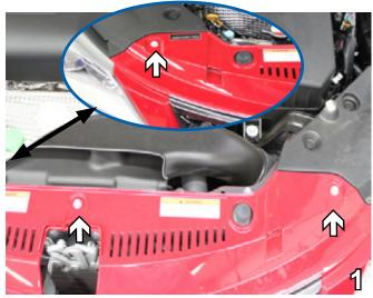
Using a 10MM socket, remove a bolt from the top of each side and the middle of the fascia. Set bolts aside to be reinstalled later.
