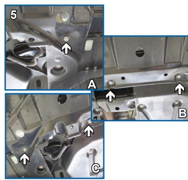
5. To remove the belly pan from the underside of the car, use a 10MM socket and remove the five bolts shown above. Set bolts and belly pan aside to be reinstalled later.
