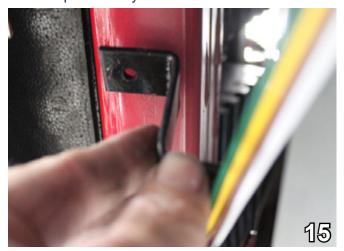
15. **Optional:** To install a breakaway switch, use a self tapping screw and attach the bracket to the bottom of the front bumper, in front of the baseplate and in between the electrical bracket and convenience link on the baseplate. Attach the breakaway to the bracket with a 1/4-20 x 3/4" hex bolt and a 1/4-20 hex nylon nut.
