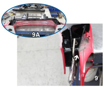
Placing the baseplate onto the bottom of the bumper and flush against it's crossbar (9A), use a clamp to secure each side of the baseplate to the bumper's legs.
