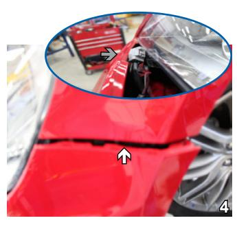
4. To remove the fascia, lift up and out on the fascia near each front tire (white arrow). To disconnect the fascia, unplug the white electrical connection located below each headlight (gray arrow). Set fascia aside to be reinstalled later.
